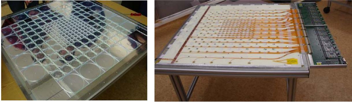
*Figure 2.1: Scintillator tile layer (left), complete module with front end electronics (right).*
