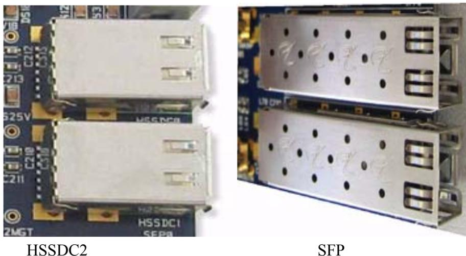
Figure 5.2. Giga-bit connector formats: HSSDC2 for (mainly) copper, SFP for fibre-optic
