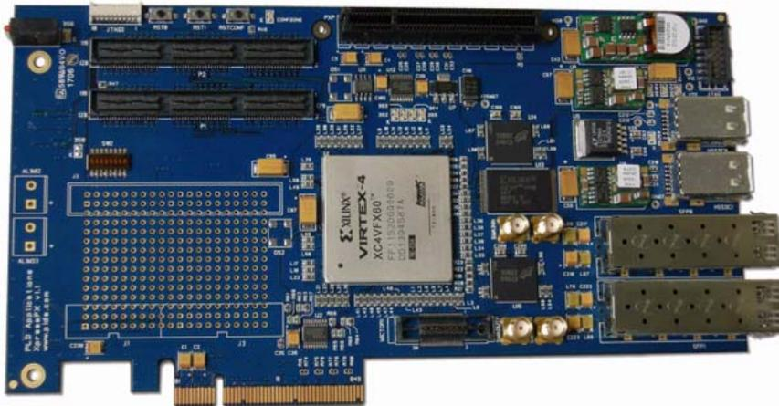
**Figure 5.4. XpressFX prototyping and development board.**
