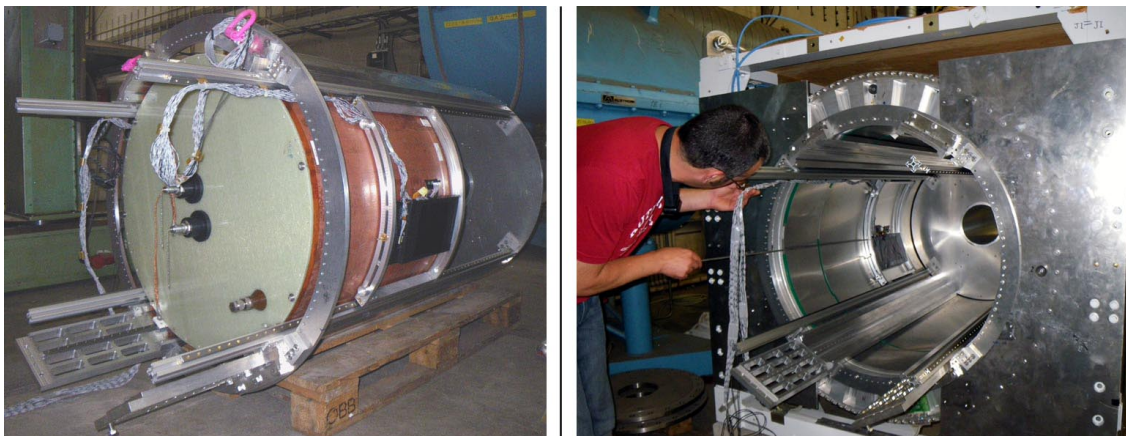
Figure 7: left: on their rails the silicon sledges can easily be moved along the TPC field cage; right: with a special pole the sledges can be positioned inside the gap between magnet and TPC
