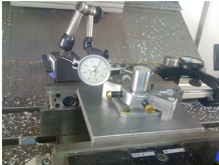
Figure 12: Prototype of the ETD quadrant fixation point fixed on the ETD end-caps.
