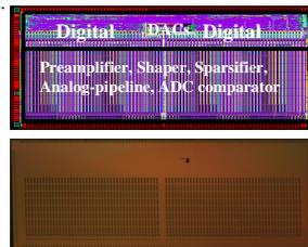
Fig. 4. The layout and photograph of the chip
