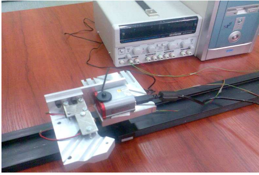
Figure 14: The test bench of the laser position monitoring system using two laser beams directed to a CCD sensor.
