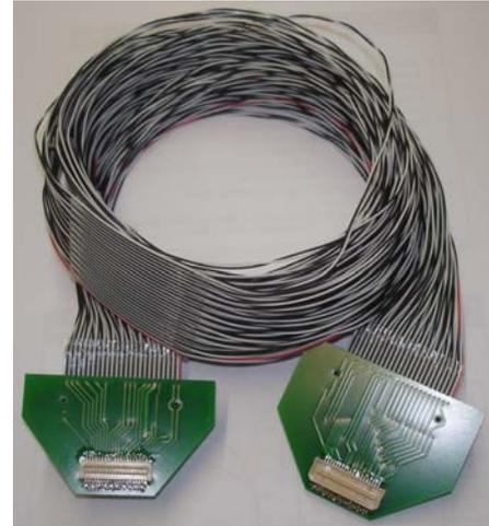
Figure 6: Schematic of the three needed adapter cards, one to connect the CMS hybrids to the twisted pair cables (left) and two for the connection of the twisted pair cables to the ICC Board (middle and right). The right photo shows two connected adapter cards.
