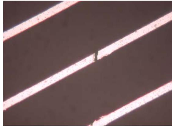
Figure 9: Such small opens in the pitch adapter lines are not easy to find. (width of the Aluminium line is 10mm)
