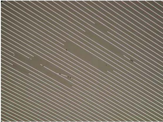
Figure 8: In the first production run problems like adhesion failures between glass and aluminium occurred.
