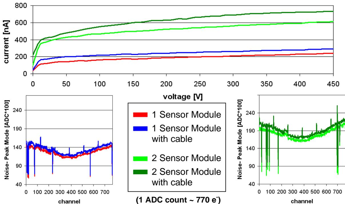
Figure 7: The top plot shows the IV curves of the two first detectors in the first built detector module, both with and without twisted pair cable. The two bottom plots show the noise of the detectors: the one sensor detector left and the two sensor detector right, again with and without cable.
