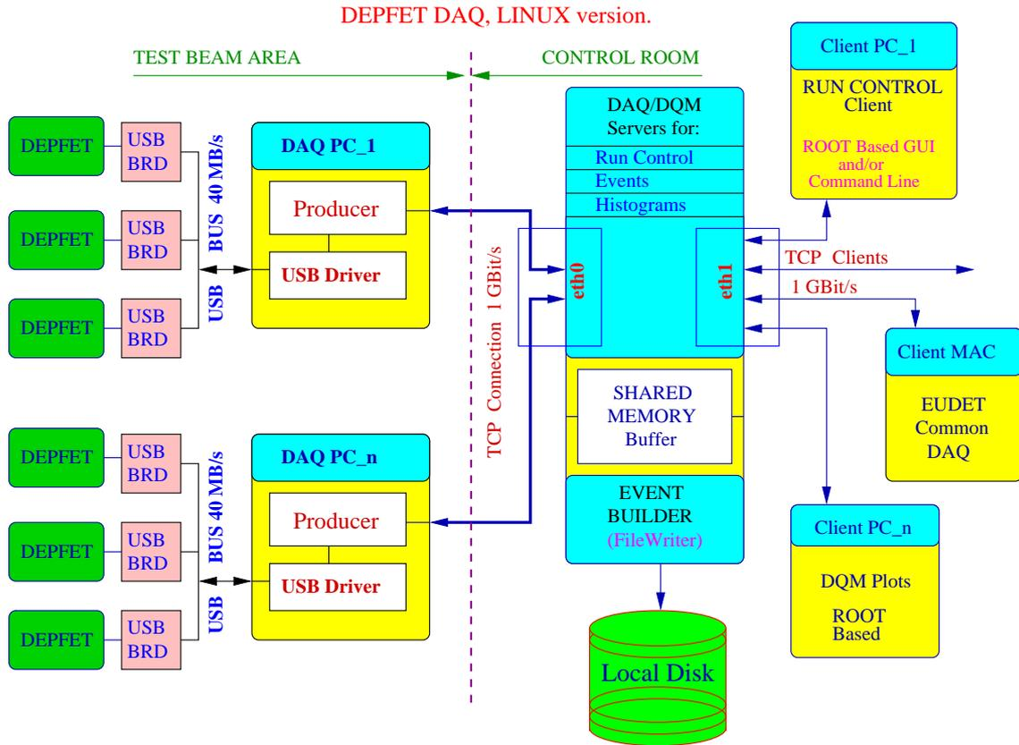
Figure 3: DEPFET Linux based data acquisition system
