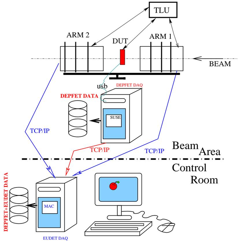
Figure 5: Test beam setup, schematic view
