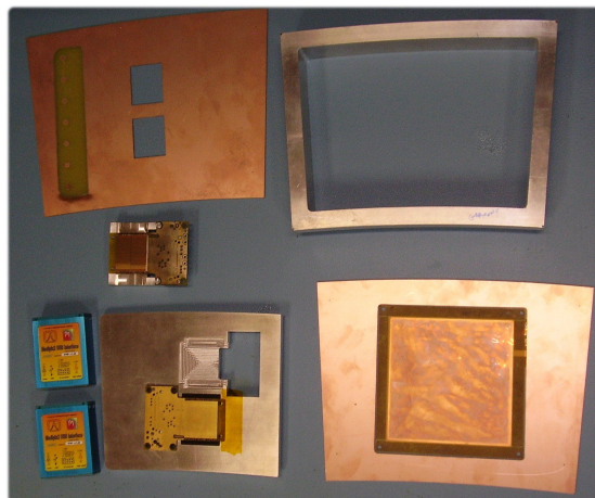
Figure 7: Readout plane, back frame, anode plane with GEM stack, reinforcement of the readout plane with one quad board (w/o chips), two USB devices, quad board with 4 Timepix ASICs (clockwise)
