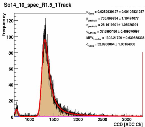
Figure 3: Sensor response with the track inside the active detector area.
