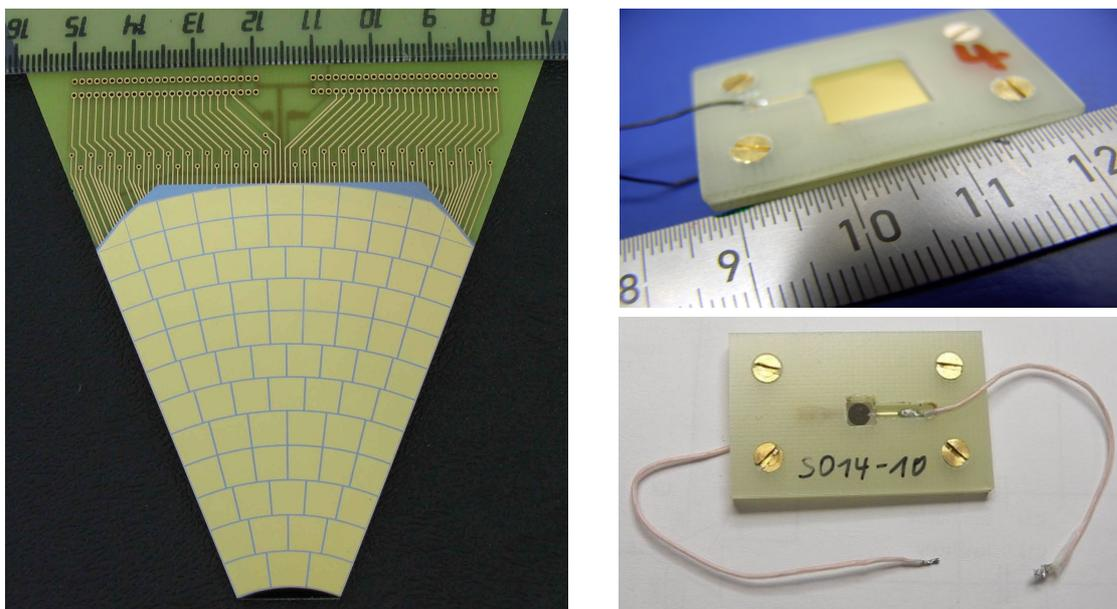
Figure 10: Examples of sensors under test. (Left): Small scale prototype of BeamCal sensor sector on the GaAs basis. (Right-top): Polycrystalline CVD Diamond detector. (Right-bottom): Single crystal CVD Diamond detector.
