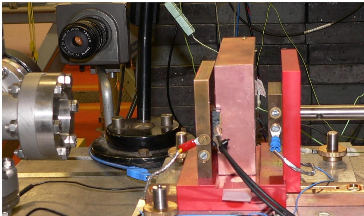
Figure 9: Equipment for radiation hardness studies at the Superconducting Darmstadt Linear Accelerator. The beam of 10 MeV electrons passes collimator, detector box and stops at the Faraday cup which is used to evaluate the absorbed dose.
