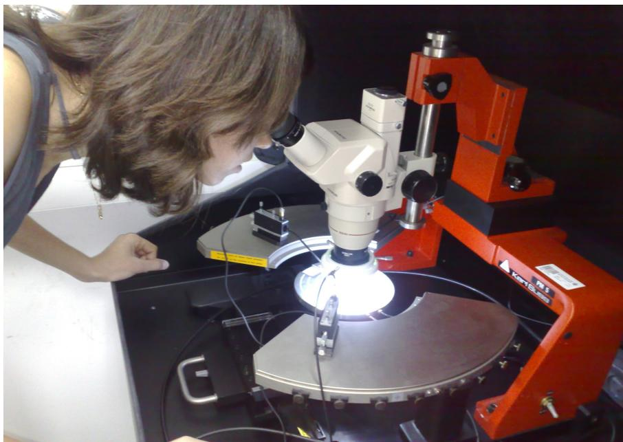
Figure 11: Computer monitored probe station at Tel Aviv University
