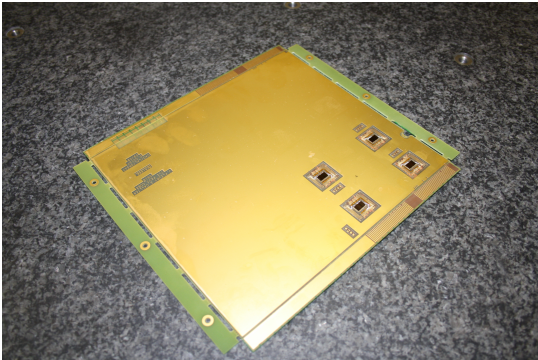
Figure 19: PCB for the CALICE SiW electromagnetic calorimeter prototype with wire bonded readout ASICs.
