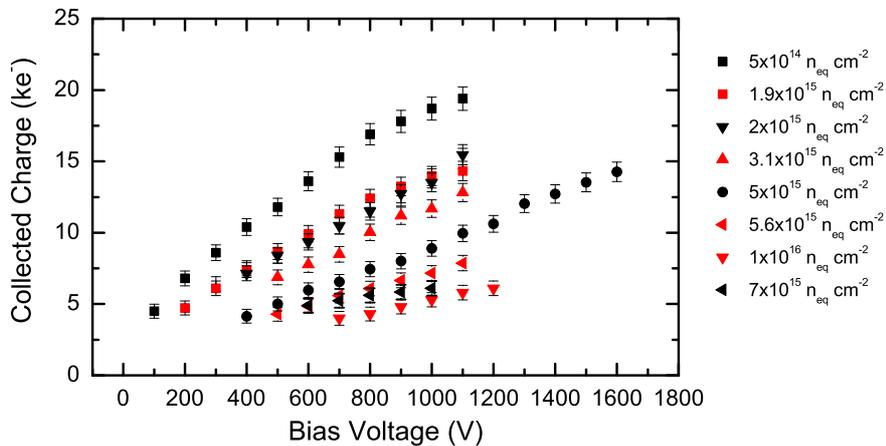
Figure 1: Collected charge for a MIP traversing a  $300 \mu\text{m}$  thick sensor as a function of bias voltage after different proton fluences [2].
