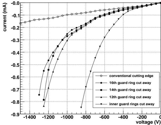
Figure 3: Leakage current characteristics of pixel sensors irradiated to  $2 \times 10^{16} \text{ n}_{eq} \text{ cm}^{-2}$  with different number of guard rings [2].
