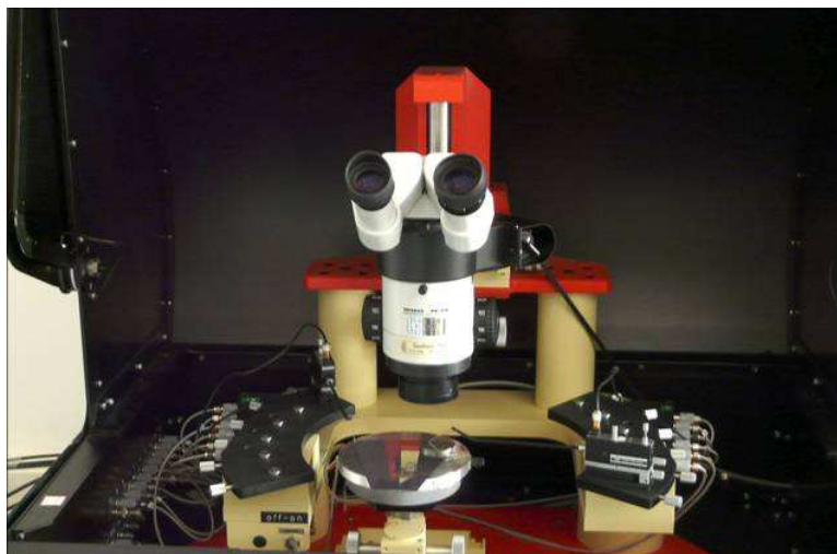
Figure 2: The prob-station foreseen for the sensor quality measurements. The device was part of the infrastructure improvement done within EUDET.
