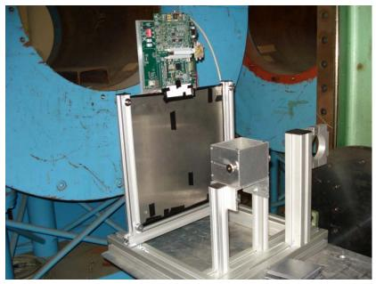
end of the segment layer, where an interface electronics collects the readout data and controls the detector's run configuration and powerpulsing.
