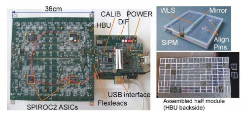
scintillating tiles each with SiPMs together with the front-end electronics and the light calibration system. The tiles are connected to the HBU's printed circuit board (PCB) by a new concept using alignment pins that are plugged into holes
