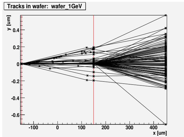
Figure 2: 100 tracks of 1 GeV electrons. The red lines represents front and the back surface of the wafer.
