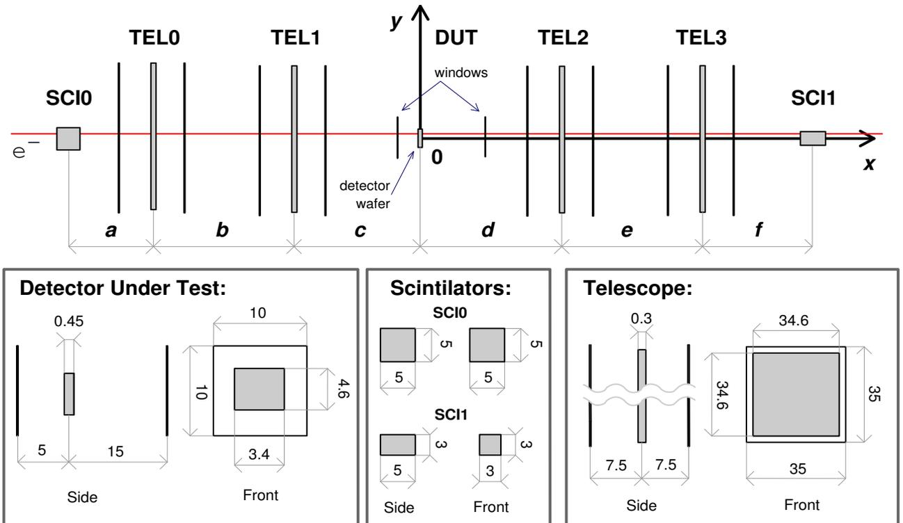
Figure 5: the geometry of the simulation. All dimensions in the figure are in millimeters.
