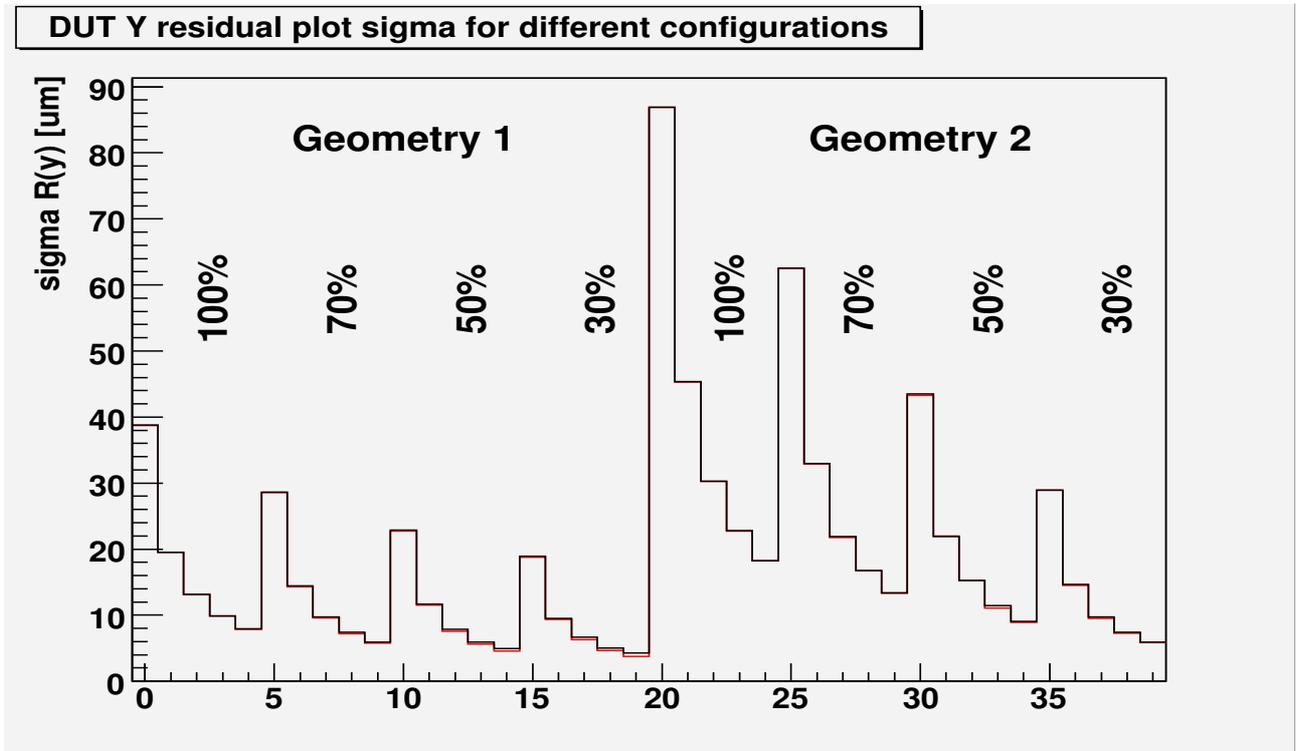
Figure 8: the comparison of the tested geometries for the electron beam. Each column represents value of the DUT residual distribution width. Groups of five columns labelled with 100% – 30% represent widths after the corresponding  $\chi^2$  cut. In each group the leftmost column corresponds to the 1 GeV electrons, the rightmost to the 5 GeV ones. The red line represents values for the ideal detectors, the black ones correspond to the simulation with the telescope intrinsic resolution included.
