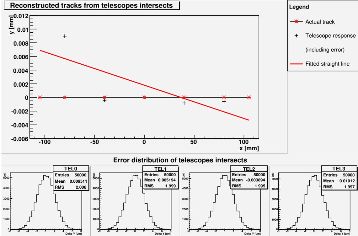
Figure 6: an example of an unscattered particle track fit in the x-y plane. The stars represents the actual intersects, the black crosses the telescopes response including the error. The residual is distance between the fitted line and the actual intersect in  $x = 0$  plane.
