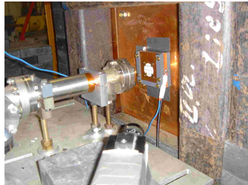
(b) Fluorescent screen mounted in a support frame and a CCD camera watching on it
