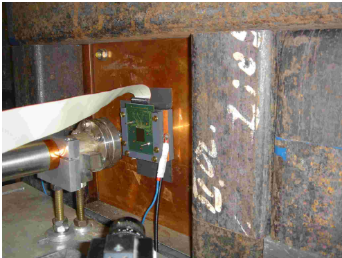
(a) MIMOSA5 chip mounted in a support frame
