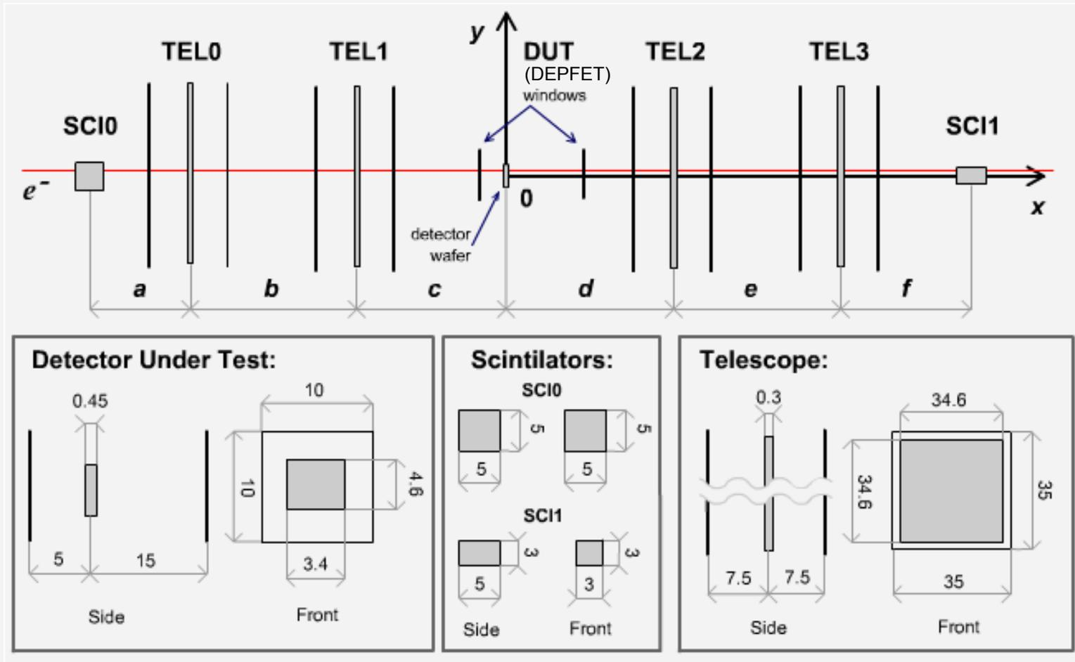
Electron beam:  $3 \times 3 \text{ mm}^2$ , homogenous, parallel with x-axis
