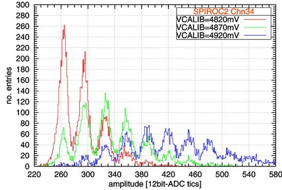
Figure 4: *Histograms of one-channel ASIC input for two LED light intensities and external triggering of the SPIROC2 ASIC. Each histogram contains about 9000 measurement entries.*
