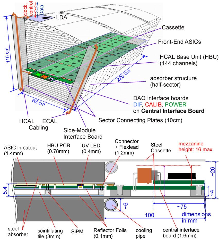
Figure 1: (top) *Electronics integration architecture for the technological AHCAL prototype.* (bottom) *Possible setup of the proposed HCAL Base Unit (HBU, cross section), showing the interface to the data acquisition modules at the endface. The numbers in brackets show the respective component heights.*
