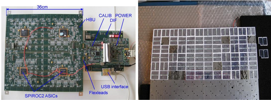
Figure 3: *Test bench set-up with the prototypes of the HBU and interfaces (left), backside of the HBU with reflector foil and tiles.*
