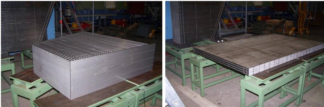
Figure 2: *The two vertical (left) and the horizontal (right) mechanical structures for the technical HCAL prototype.*
