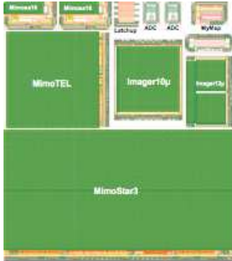
Figure 2: The MIMO TEL sensor and the high resolution sensor HRT (called Imager10 \mu here) on the wafer layout.
