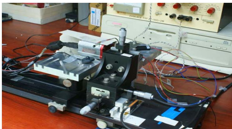
Figure 2. The laboratory setup used in tests of the laser positioning system.
