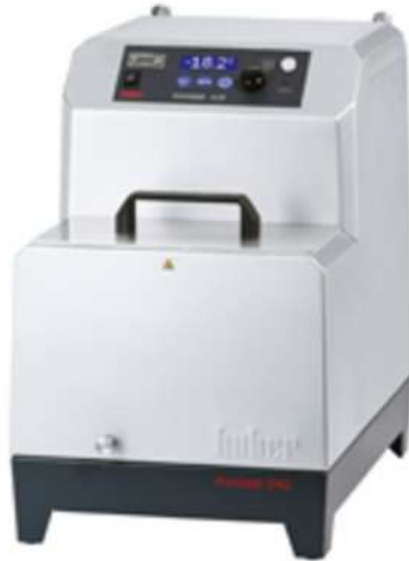
Figure 6: Photograph of the cooling device Huber ministat 230-4.
