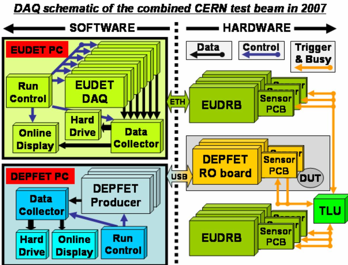
Figure 2: Schematic of the DEPFET and EUDET telescope DAQ integration during the CERN test beam season in 2007: The right side covers the hardware with 2 DEPFET DUT and 6 EUDET telescope planes. Event synchronization is done by a trigger logic unit (*TLU*) with a trigger-busy handshake protocol and a transmission of an individual trigger number for each event to all modules. The left side shows the software structure: Two separated DAQ systems were running on two PC.
