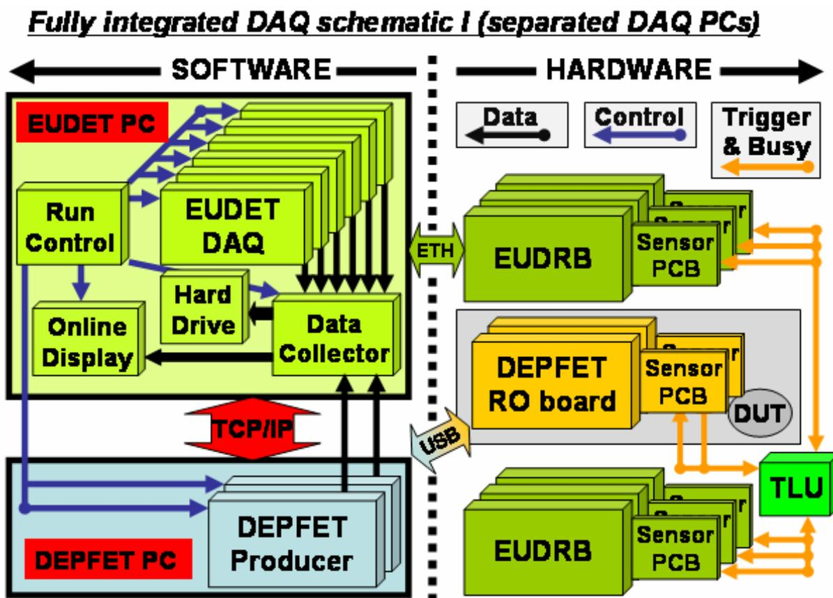
Figure 6: Schematic of running a common DAQ on two separate PC. The DUT *producer* receives start and stop commands from the *run control* and sends its data to a memory block. This memory block is accessed by the *data collector* for event building. A common *online monitoring* is feed by the *data collector*. The PC are linked via a high speed Ethernet TCP/IP network.
