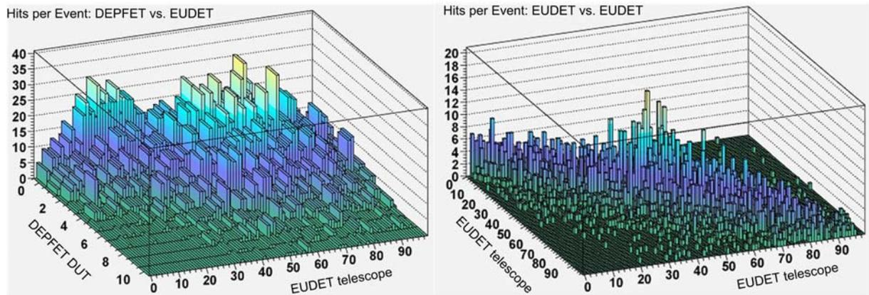
Figure 3: The event multiplicity distribution of a DEPFET DUT vs. a EUDET telescope plane 3 (left image) and telescope plane 2 vs. telescope plane 3 (right image).
