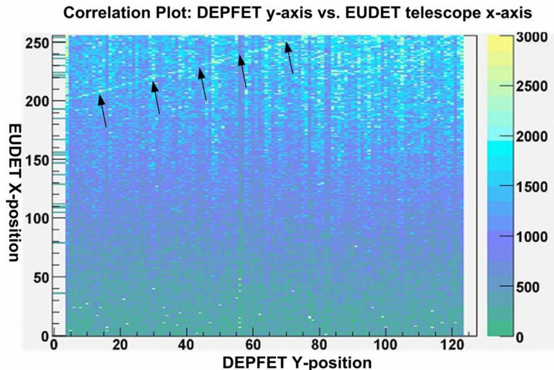
Figure 5: Correlation of hit positions of the y-axis of the DEPFET DUT vs. the x-axis of the EUDET telescope plane 2. The sensors are tilted by 90° with respect to each other. Due to the high hit multiplicity the background is very large. The correlation reveals that the DUT is only partially covered along this axis.
