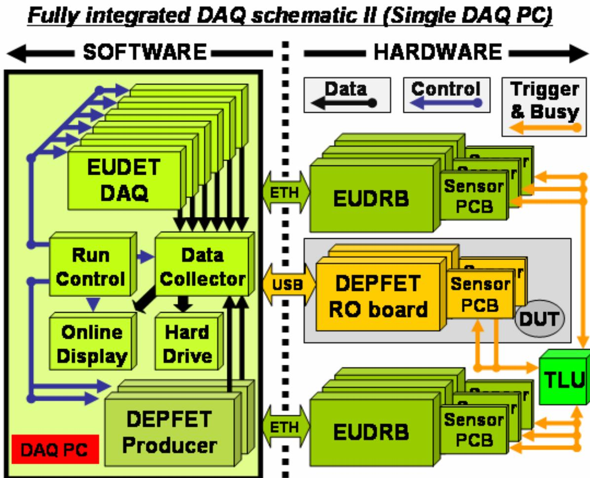
Figure 7: Schematic of running a common DAQ on two separated PC. The *DUT producer* receives start and stop commands from the *run control* and sends its data to a memory block. This memory block is accessed by the *data collector* for event building. A common online monitoring is fed by the *data collector*.
