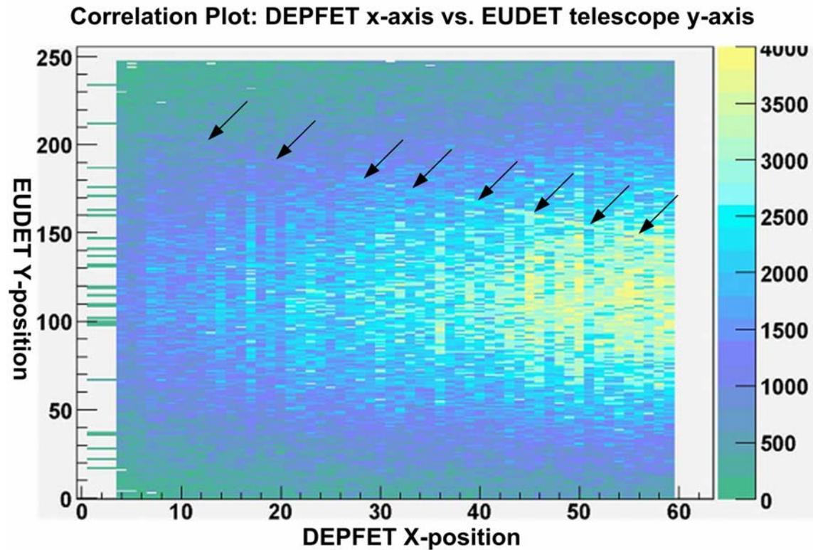
Figure 4: Correlation of hit positions of the x-axis of the DEPFET DUT vs. the y-axis of the EUDET telescope plane 2. The sensors are tilted by 90° with respect to each other. Due to the high hit multiplicity the background is very large, but the correlation reveals a full coverage of the DEPFET DUT for this axis.
