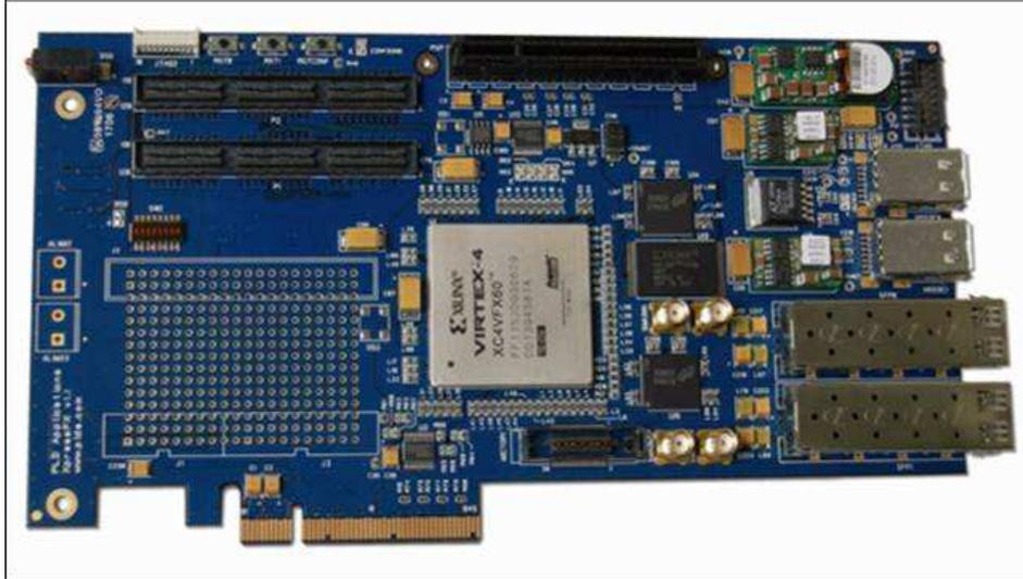
Figure 6: The PLDA V4FX100 FPGA hardware development platform for the ODR.
