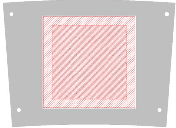
Figure 7: Drawing of the electrical shield holding the GEMs for the LP module.
