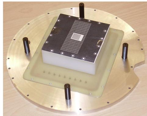
Figure 5: A paper printout of the combined pads + TimePix readout plane mounted on the readout back frame.
