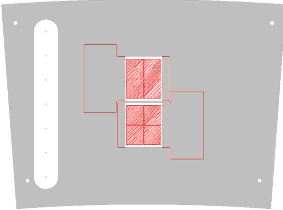
Figure 6: Sketch of the LP module's readout plane. On the left side one can see the high voltage feed through. In the middle the shapes of the two quad boards with the TimePix chips are indicated. The quad boards will be glued in from the back side.
