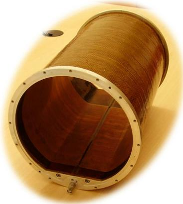
Figure 2: The prototype field cage.
