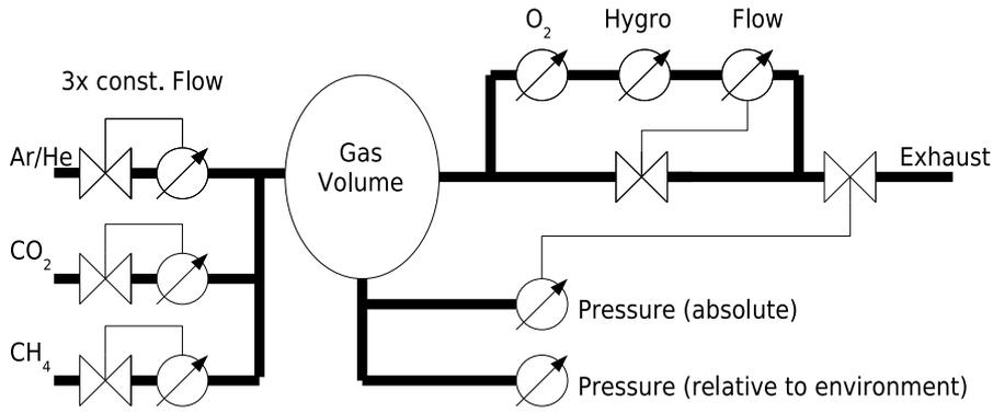
Figure 1: The planned gas system for the test setup.
