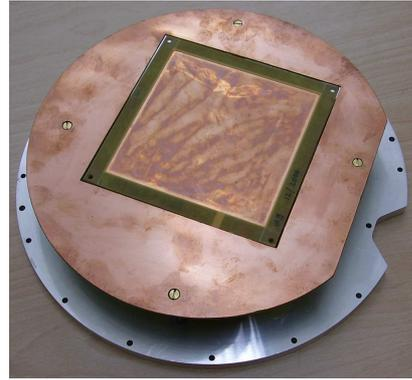
Figure 3: The electrical shield with a GEM mounted in it.
