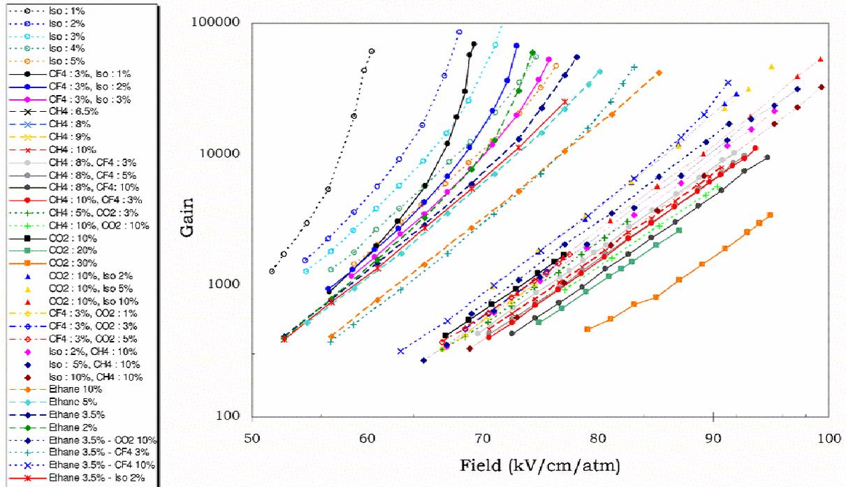
Figure 1: Gain curves vs. amplification field measured by a Micromegas detector using gas mixtures containing Argon and a few percent of CO<sub>2</sub>, CH<sub>4</sub>, C<sub>2</sub>H<sub>6</sub>, Iso-C<sub>4</sub>H<sub>10</sub>, and CF<sub>4</sub>.
