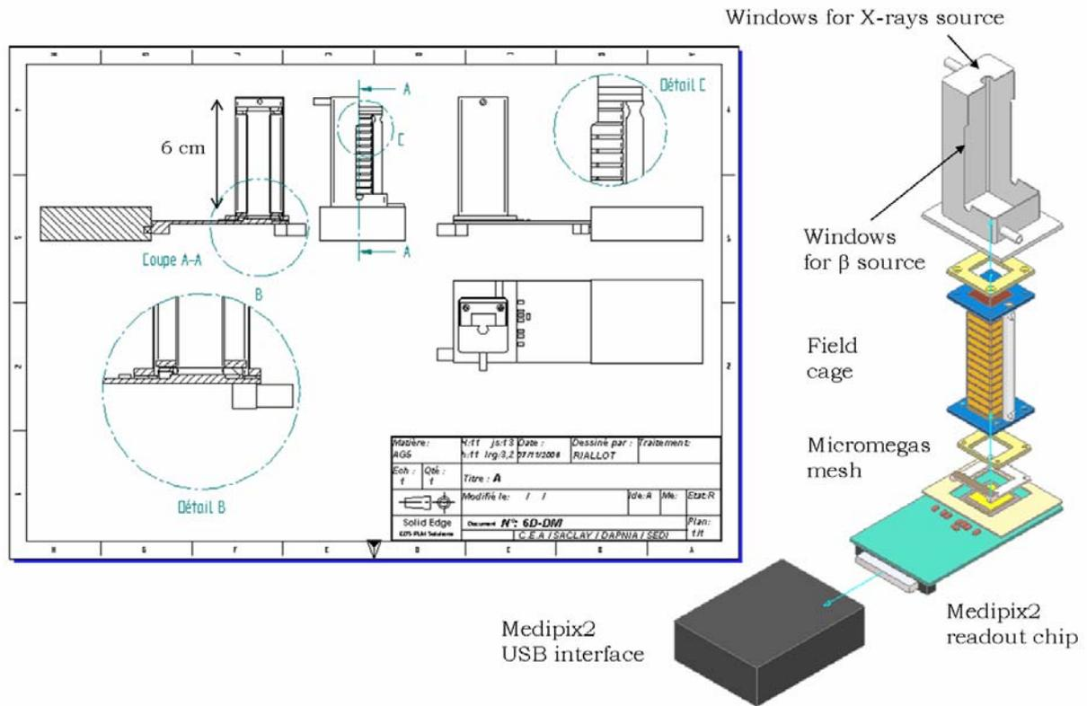
Figure 4: Design for a small chamber with a Micromegas mesh built inside and placed above the PCB of Medipix2/TimePix readout chip.
