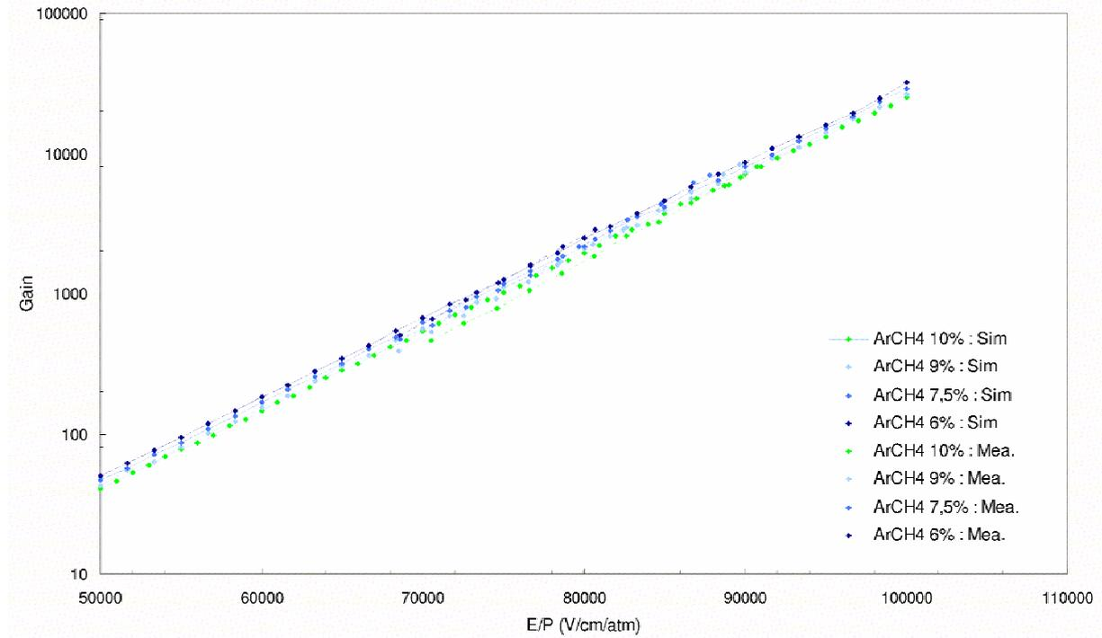
Figure 2: Simulated and measured gain as a function of the electric fields E for Ar/CH<sub>4</sub> at several percentages.
