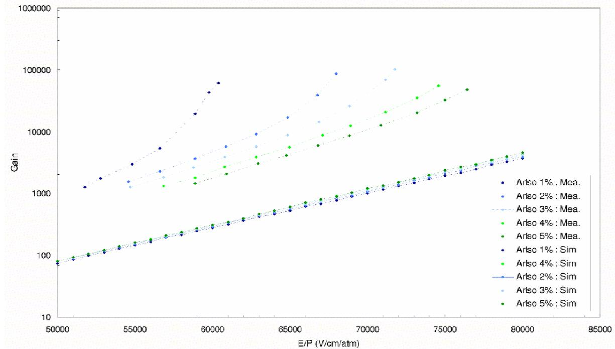
Figure 3: Simulated and measured gain as a function of the electric fields E for Ar/C<sub>4</sub>H<sub>10</sub> at several percentages.
