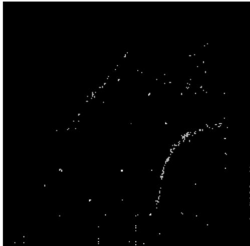
*Figure 1: Track of a cosmic particle going through a  $1 \text{ cm}^3$  volume of Helium Isobutane 80/20.*
