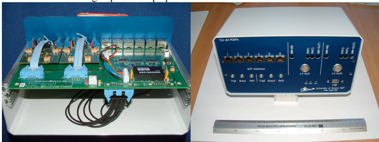
Figure 6: The motherboard of the TLU inside the box and the assembled box (without PMT daughter boards)
