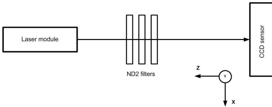
Fig.1. The setup for the transversal (x, y) displacement measurement with single laser beam.
