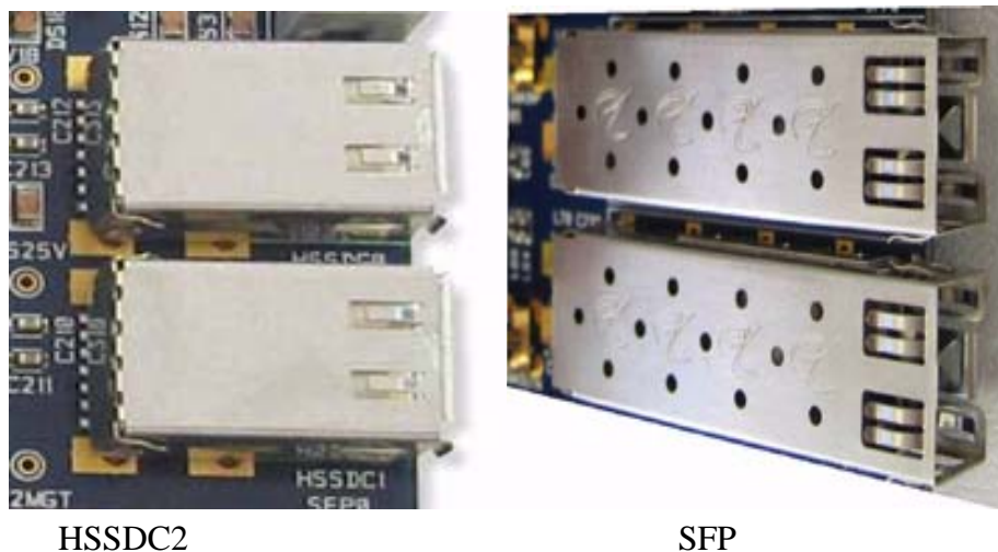
Figure 2. Giga-bit connector formats: HSSDC2 for (mainly) copper, SFP for fibre-optic
