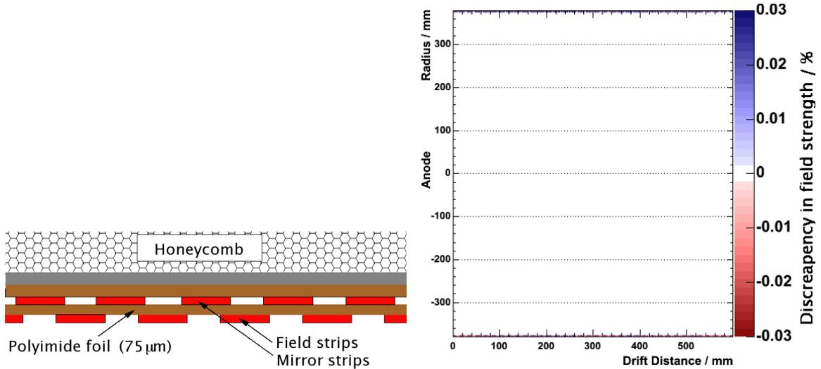
Figure 7: Layout and field map for a design with two layers of field strips (width of the strips 2.3 mm and of the gaps 0.5 mm) for the LP
