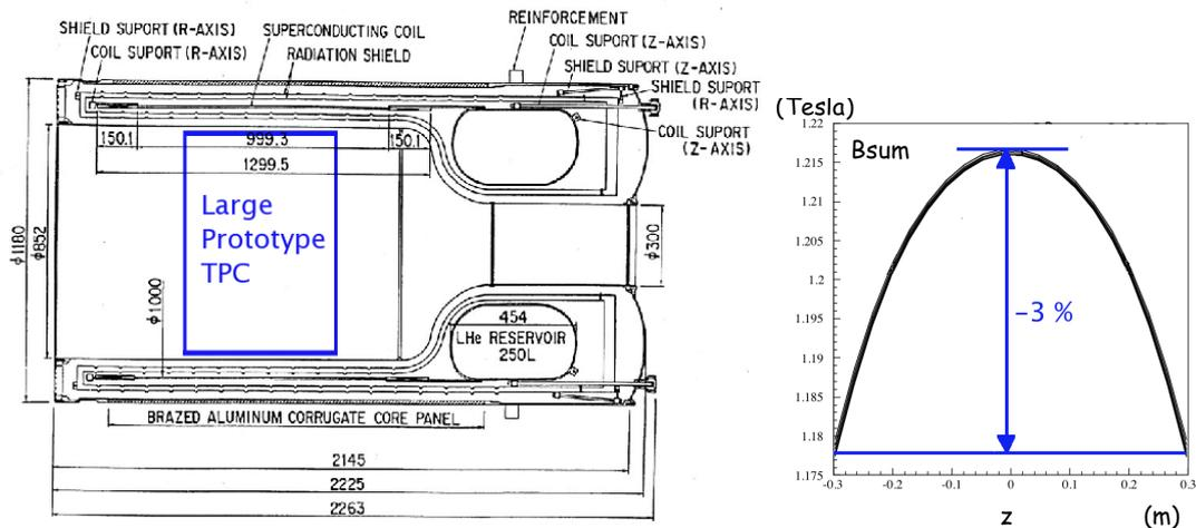
Figure 1: Technical drawing of the PCMAG (from [KEK]) and the result of a magnetic field calculation on the axis of the magnet (from [PCM])
