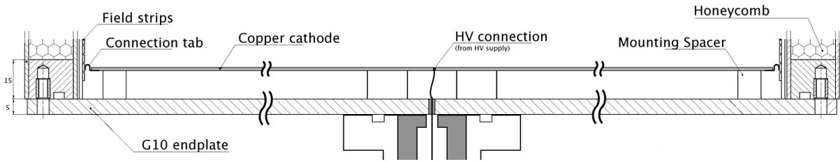
Figure 3: Cathode mounted to the endplate
