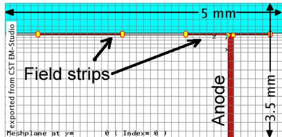
Figure 5: Cutout of the model set up for the drift field calculations
