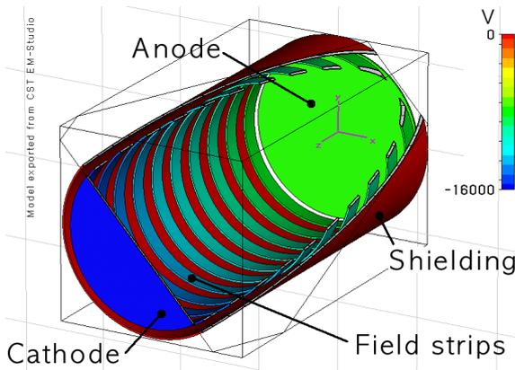
Figure 4: Schematic design of a cylindrical TPC
