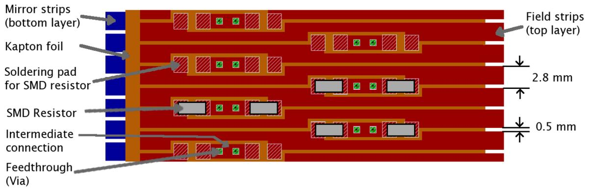
Figure 8: Design of the foil field-strip foil
