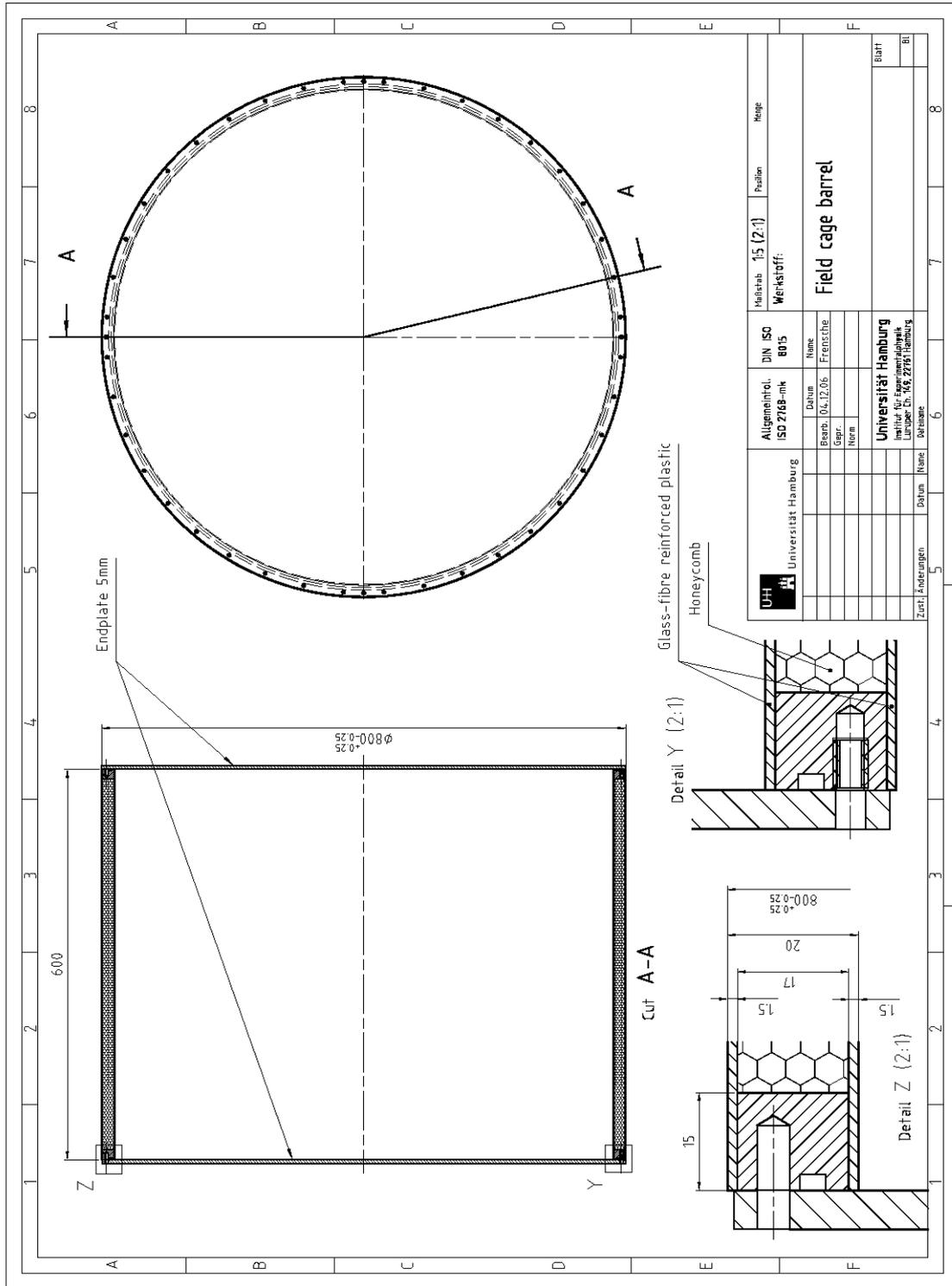
Figure 2: First iteration of construction plans for the field cage barrel
