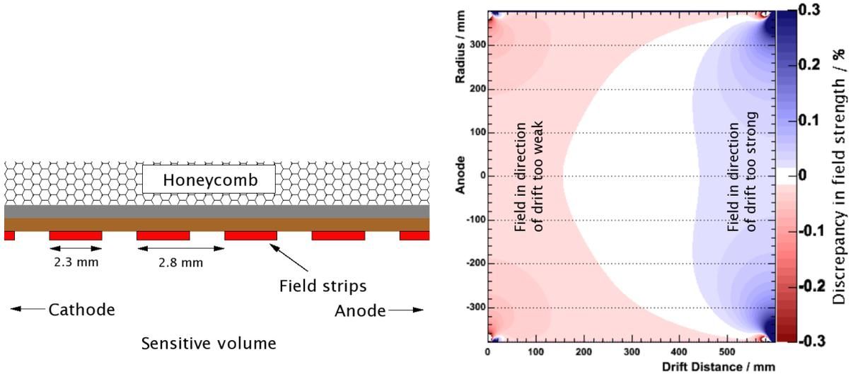
Figure 6: Layout and field map for one-sided field strips of 2.3 mm width and 0.5 mm gaps
