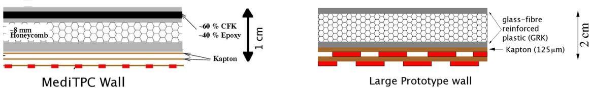
Figure 11: Comparison between the profiles of the MediTPC wall (from [Lux]) and the proposed wall of the LP
