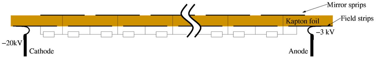
Figure 10: Circuit plan for the connection of the field strips
