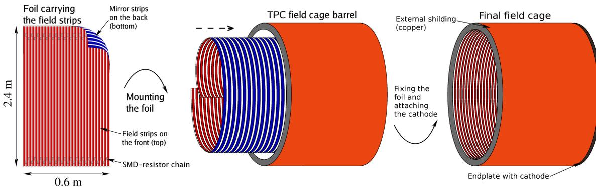
Figure 12: Mounting the field-strip foil into the field cage barrel
