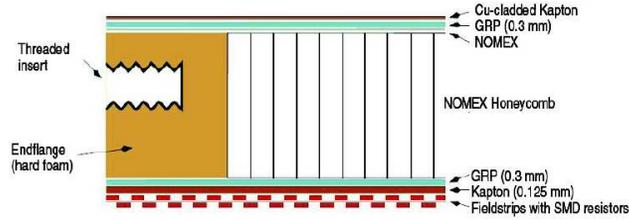
Figure 2: Sandwiched structure for the field-cage.
