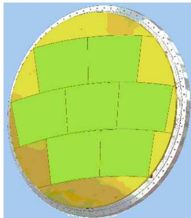
Figure 6: Anode end plate with amplification modules and termination plates.
