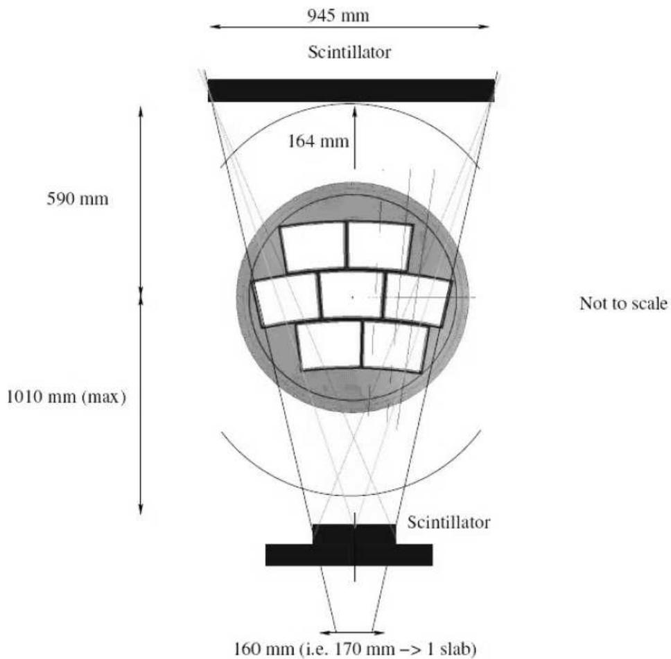
Figure 10: Scintillator hodoscope setup with the LP TPC. The central disk depicts the end plate of the TPC.
