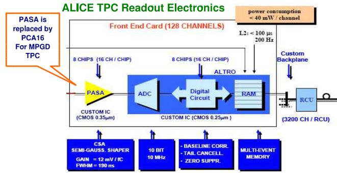
Figure 3: Schematics of the ALTRO electronics. The PASA chip has been replaced by the PCA16 chip. The AFTER electronics which will be used for the MicroMegas modules have a similar setup.
