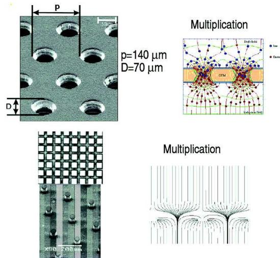
Figure 7: MPGD techniques. Upper: GEM, lower: MicroMegas.
