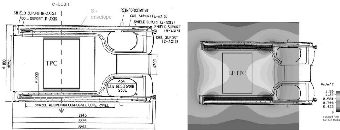
Figure 11: Schematic drawing of PCMAG and its field density distribution.
