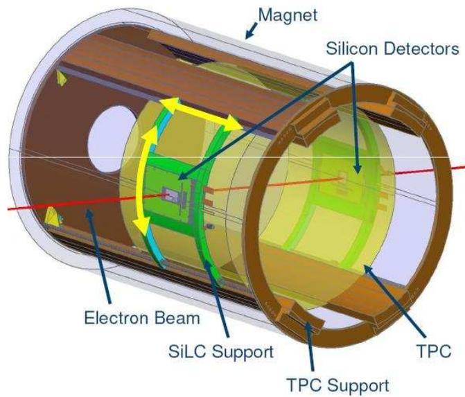
Figure 5: Silicon detectors which are mounted on a support structure around the LP.
