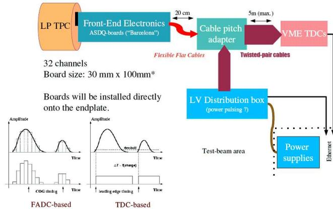
Figure 4: Schematics of a TDC based electronics.
