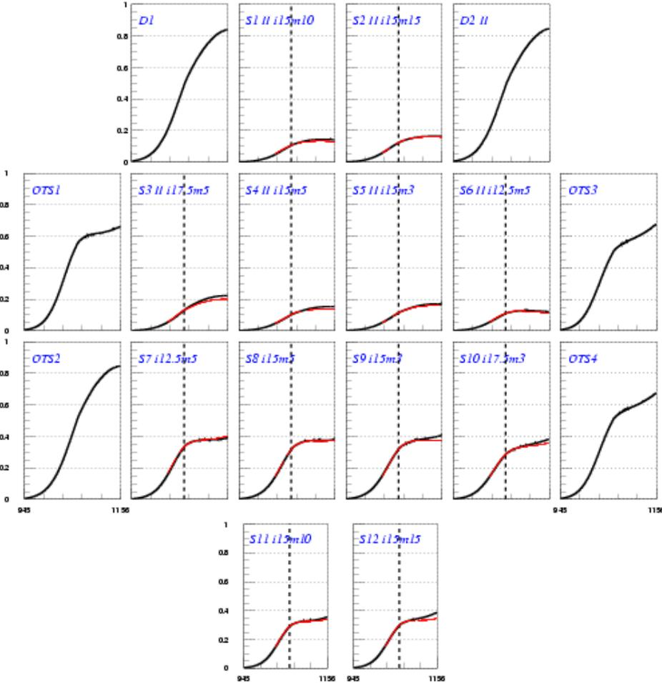
Figure 5: Measured transmittance (black) and calculated (red) for the 12 sensors of the wafer
