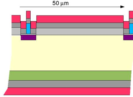
Figure 3: *Standard ILC baseline strip sensor cross section. Same color code as the figure in the left. Dimensions are not scaled.*
