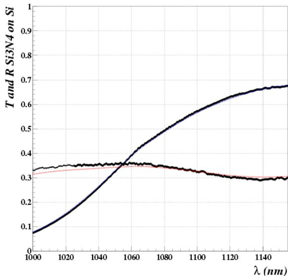
Figure 6: Measured transmittance (black, slanted line) and reflectance (black trace, horizontal) of a  $1\ \mu\text{m}$  thick layer of  $\text{Si}_3\text{N}_4$  on Silicon, compared to calculation. Blue graph for transmittance, red for reflectance.
