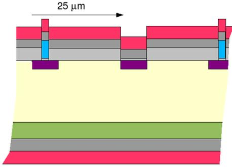
Figure 2: *Cross section of a sensor with an intermediate implant, 25  $\mu\text{m}$  away from a readout electrode. Color code: red for nitride, gray for silicon dioxide, violet (green) for p (n) implant, yellow for Si. Not to scale*
