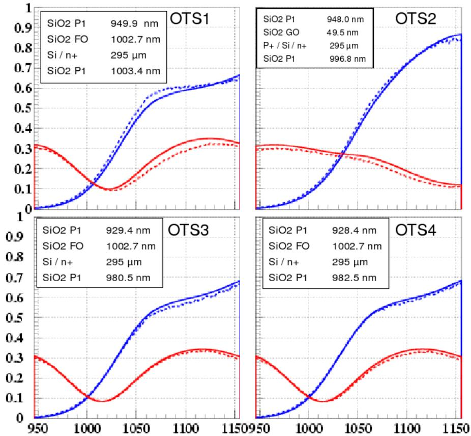
Figure 4: Measured transmittance (dashed line, blue) and reflectance (red) of the 4 OTS (ordinates axis) versus wavelength (in abscissas) compared to calculation (continuous lines).
