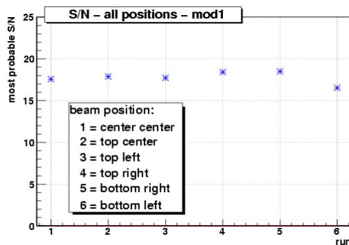
Figure 7: SNR measured with particles in the center of the detector (point 1) without Al, compared to the areas around the alignment passage.
