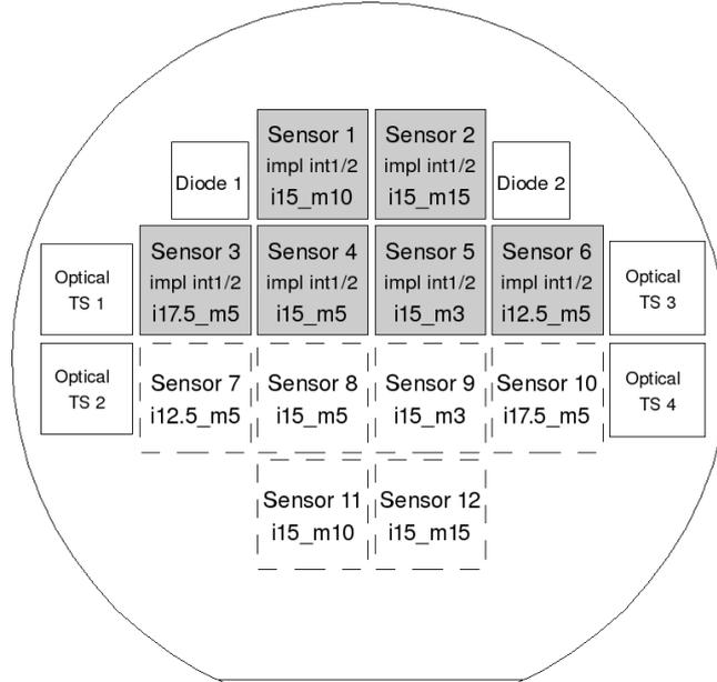
Figure 1: Overview of the sensor arrangement in the wafers. Sensors are labeled in increasing order, from top left to right bottom.
