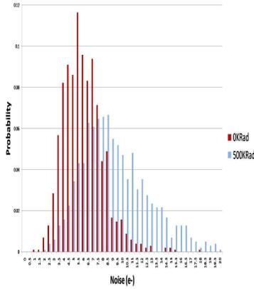
Figure 6: Noise distributions measured before irradiation and after 500 kRad.
