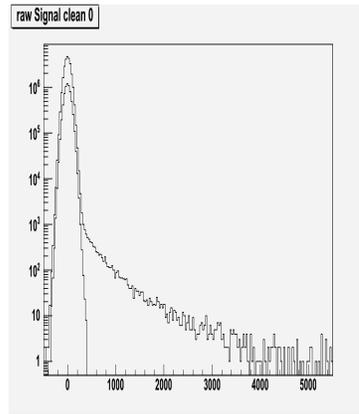
Figure 11: Pedestal corrected signal for each pixel in each event with and without beam.
