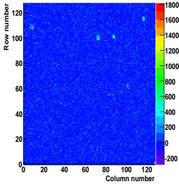
Figure 10: Event display taken with a high resistivity FORTIS 1.1. Five hits can clearly be seen.
