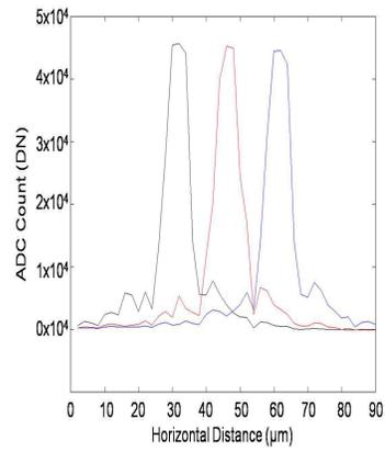
Figure 9: Laser scan using a FORTIS 1.1. with a high resistivity epitaxial layer
