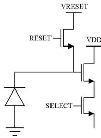
Figure 1: 3T CMOS pixel architecture
