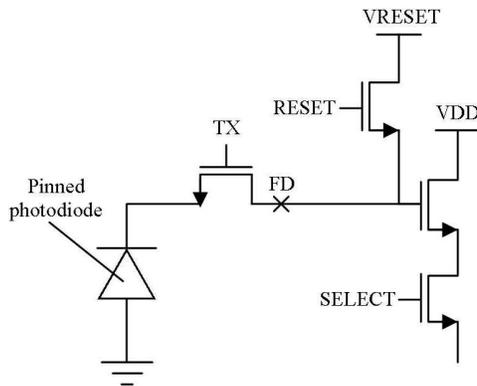
Figure 2: Advanced 4T CMOS pixel architecture
