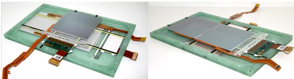
Figure 4: Open detector module with the one-sensor detector on top (left) and the two-sensor detector on top (right)
