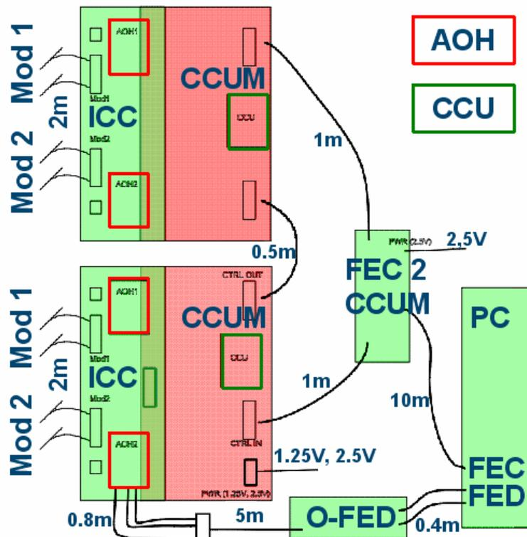
Figure 12: Schematic of the adopted CMS Tracker Readout System
