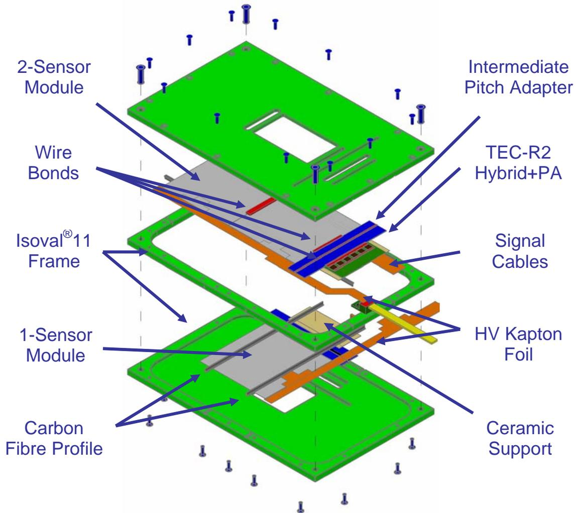
Figure 2: Exploded Drawing of a silicon detector
