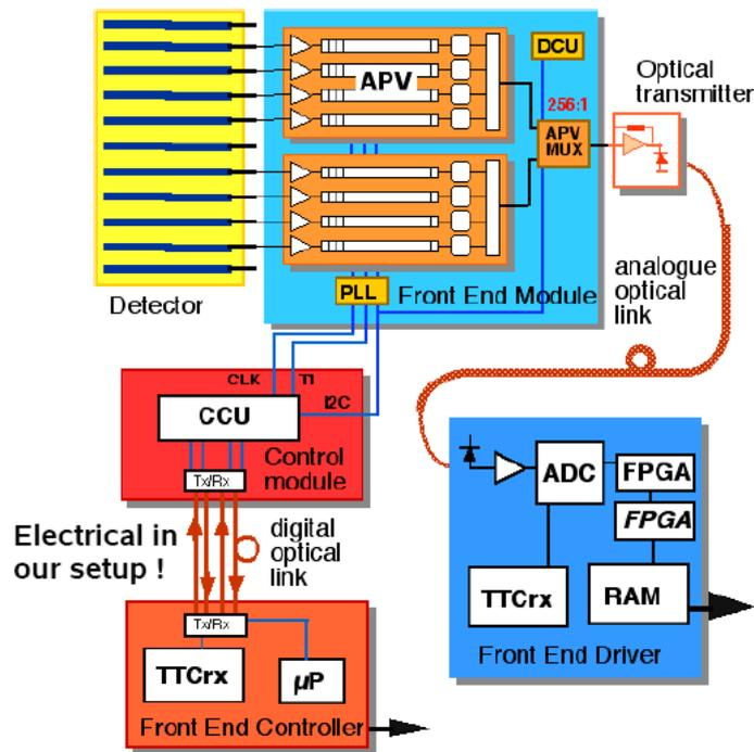
Figure 11: Schematic of the CMS Tracker Readout System
