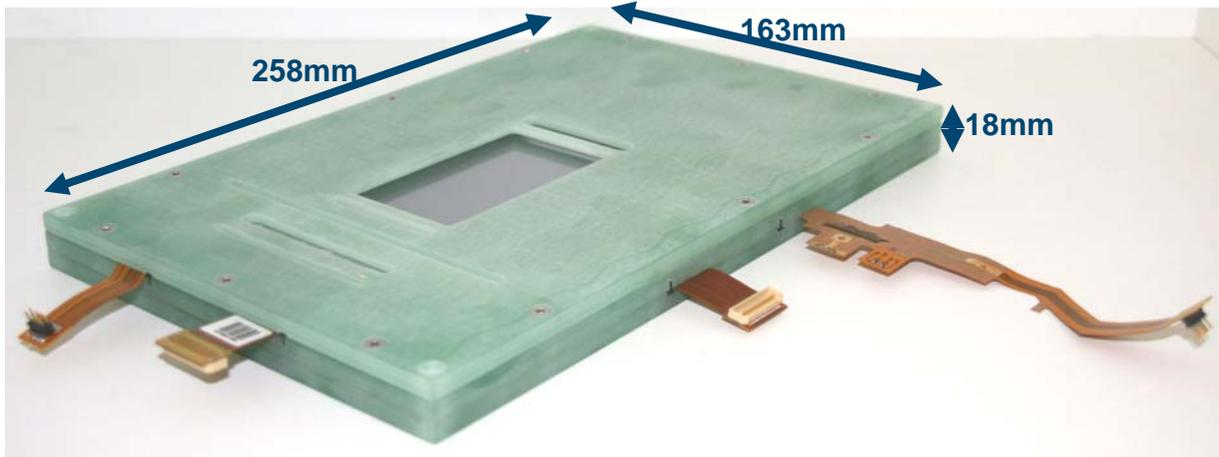
Figure 3: Closed silicon detector module (without light-tight adhesive foil)
