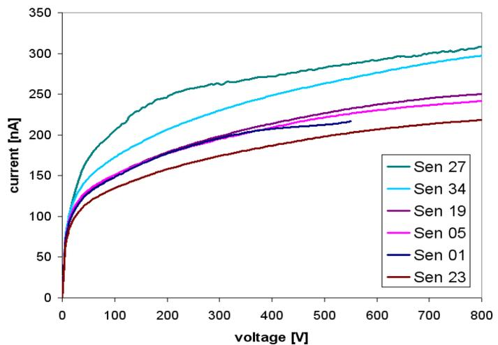
Figure 5: The table displays the depletion voltage (Vdepl) and the leakage current at 300 V (I300V) and 400 V (I400V) of the six sensors. The plot shows the IV-curves of these sensors.
