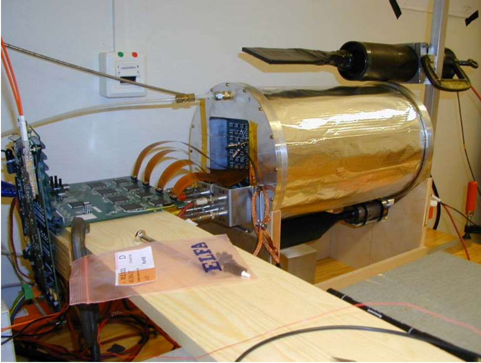
Fig 8. Photograph of the cosmic setup with a TPC and one FEC+RCU for readout.
