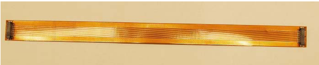
Fig 6. A photograph of a 30cm long Kapton cable.
