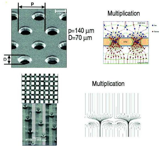
Figure 3: MPGD techniques. Upper: GEM, lower: Micromegas.
