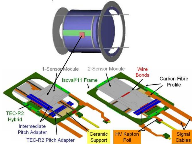
Figure 8: Silicon detectors which are mounted on a support structure around the LP.
