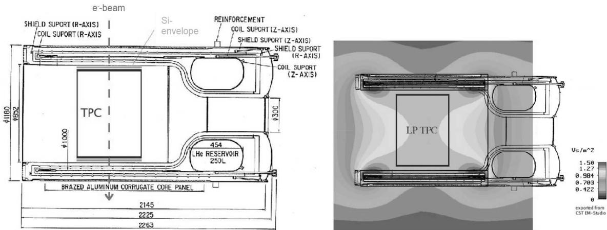
Figure 9: Schematic drawing of PCMAG and its field density distribution.
