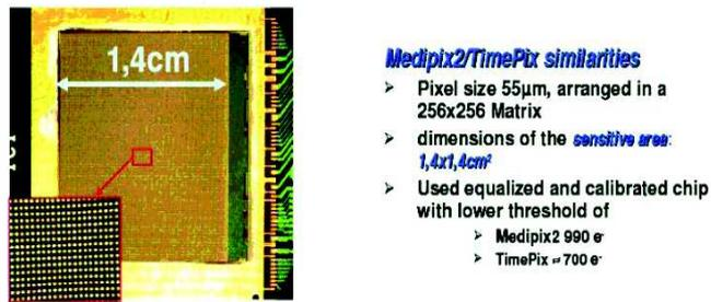
Figure 4: MediPix readout technique.
