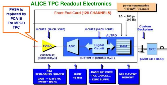
Figure 6: Schematics of the ALTRO electronics. The PASA chip will be replaced by the PCA16 chip. The AFTER electronics which will be used for the Micromegas modules have a similar setup.
