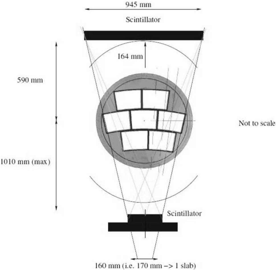
Figure 11: Scintillator hodoscope setup with the LP TPC. The central disk depicts the end plate of the TPC.
