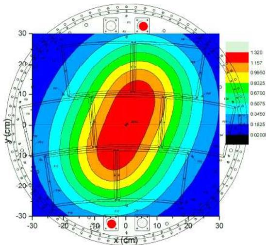
Figure 5: Charge distribution on the anode of a photoelectron calibration system.
