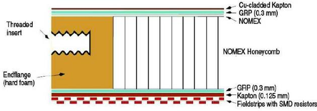
Figure 1: Sandwiched structure for the field-cage.
