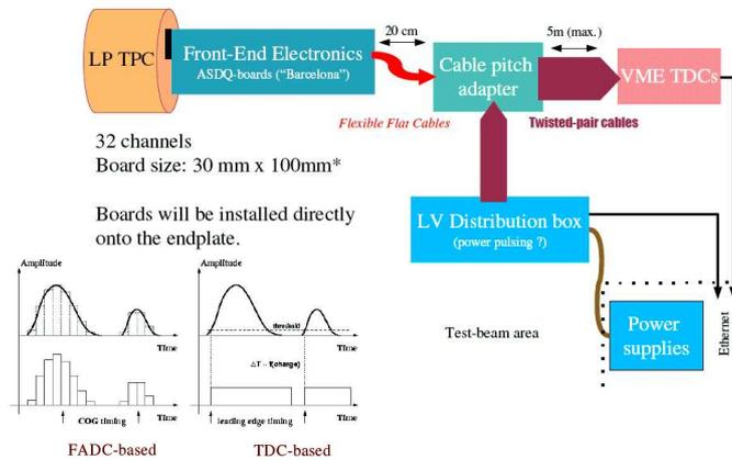
Figure 7: Schematics of a TDC based electronics.
