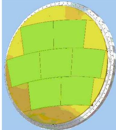
Figure 2: Anode endplate with amplification modules and termination plates.
