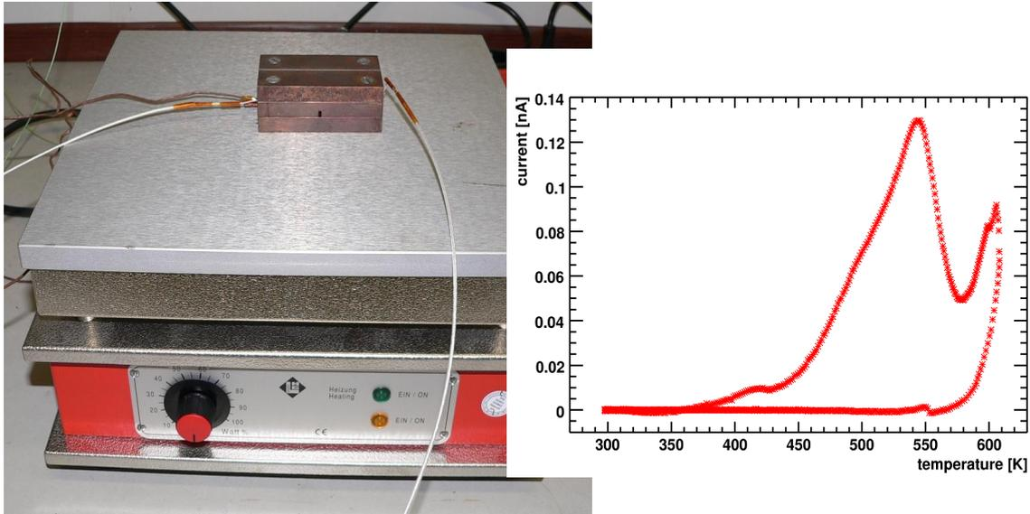
Figure 8: Setup for measurements of Thermally Stimulated Current (TSC). In the inset the typical dependence of TSC on temperature is shown for radiation damaged diamond detector.
