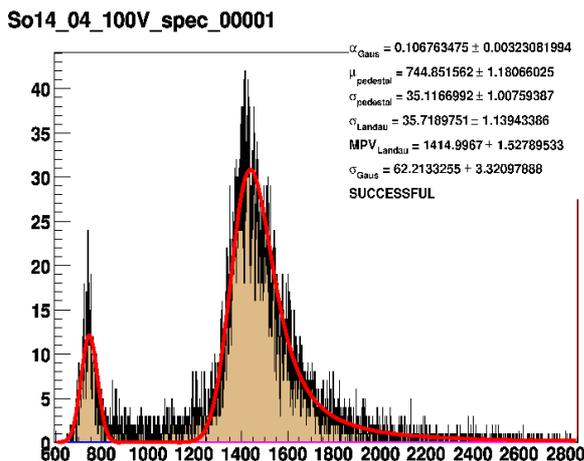
Figure 6: Single crystal diamond spectrum before the upgrade.
