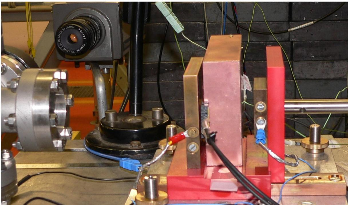
Figure 9: Equipment for radiation hardness studies at the Superconducting Darmstadt Linear Accelerator. The beam of 10 MeV electrons passes collimator, detector box and stops at the Faraday cup which is used to evaluate the absorbed dose.
