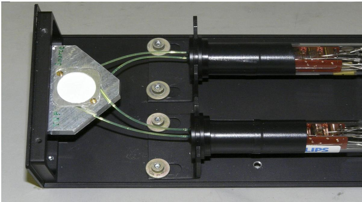
Figure 5: New trigger counters for  $^{90}\text{Sr}$  setup. Counters are mounted in the metal holder and covered by thin reflective TYVEK paper. The light is readout by helix-like WLS fibres and registered by photo-multipliers. Light-tight cover of the box (not shown) has a thin entrance window above the counters.
