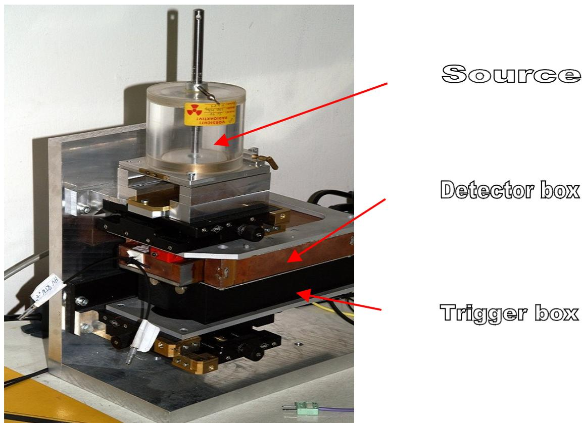
Figure 4: Experimental setup at DESY-Zeuthen for detector CCE measurements using  $^{90}\text{Sr}$  source. The box, containing the detector under test and trigger counter box are placed onto adjustable XY-supports for the precise alignment.
