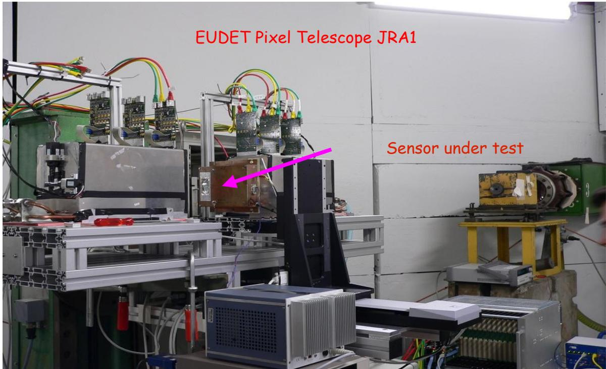
Figure1: Experimental setup at the DESY-Hamburg testbeam. The detector under study is placed in the beam line between two arms of the EUDET telescope.
