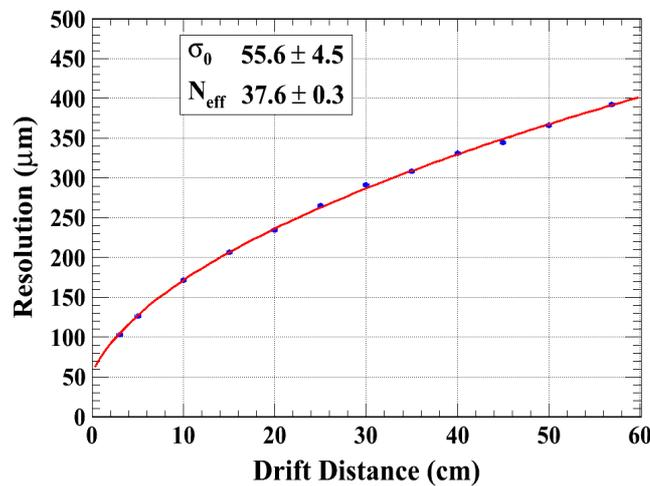
Figure 6. Measured resolution as a function of drift distance Z for module 4 at B=0 T.
