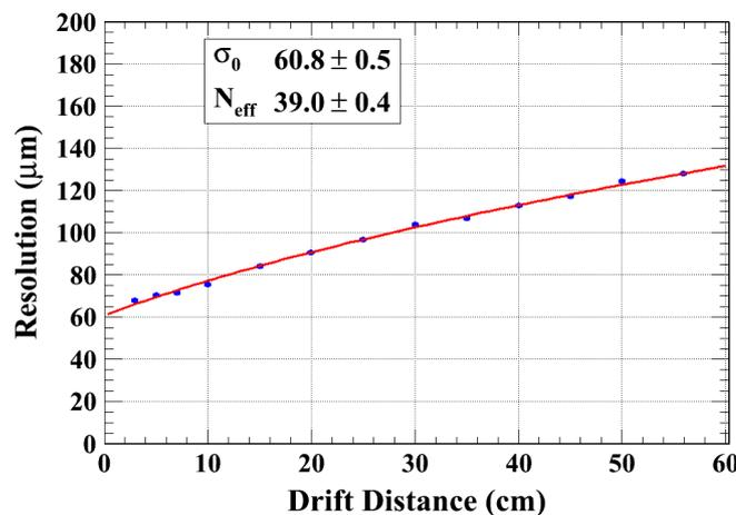
Figure 7. Measured resolution as a function of drift distance Z for module 3 at B=1 T.
