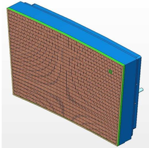
Figure 3. The Micromegas detector module (24 pad rows  $\times$  72 columns).
