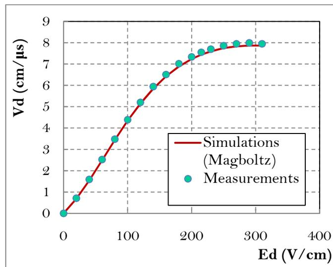
Figure 4. Drift velocity measurements ( $B=0T$ ).
