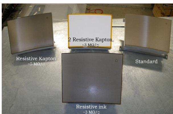
Figure 1. The five Bulk Micromegas detector modules.
