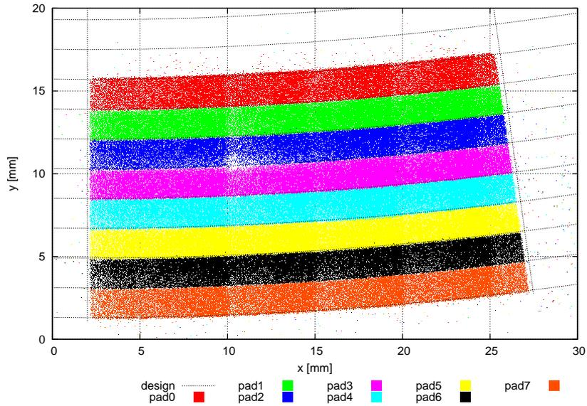
Figure 6: Reconstructed position of beam particle impact point combined with signals registered in LumiCal sensor pads.
