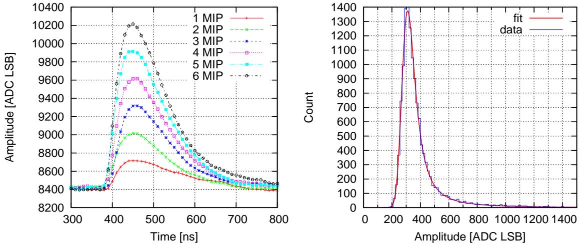
Figure 4: Time response for different energy depositions (left) and energy deposition distribution in single channel (right).
