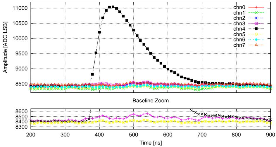
Figure 5: Response of 8 channels under test to particle passing through channel 4 (top) and baseline zoom of neighbours channels (bottom)
