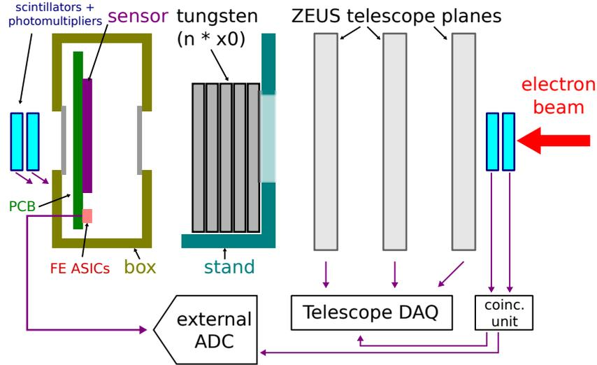
Figure 2: Experimental setup used during beam test measurements.
