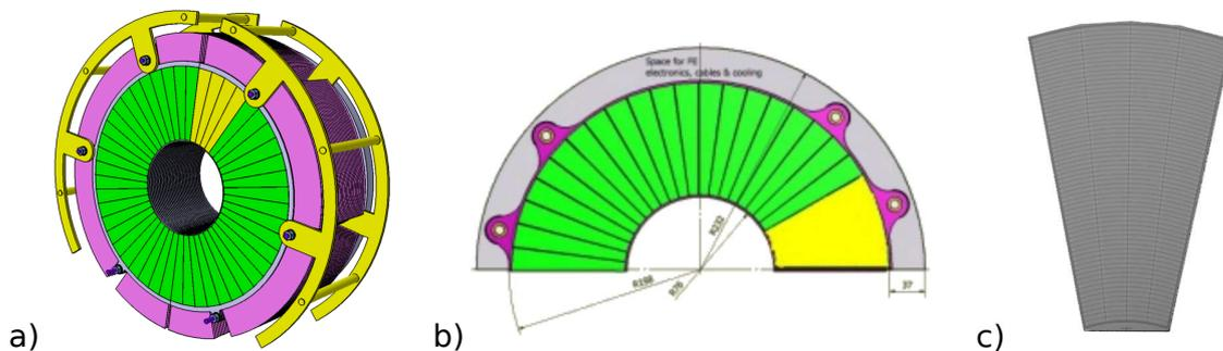
Figure 1: a) LumiCal calorimeter design b) Half plane, silicon sensor tail marked on yellow c) Silicon sensor tail prototype used during test beam measurements together with dedicated front-end electronics.
