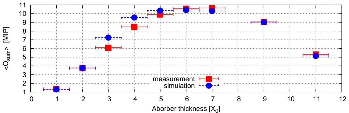
Figure 8: Average charge deposited in instrumented area as a function of tungsten thickness.
