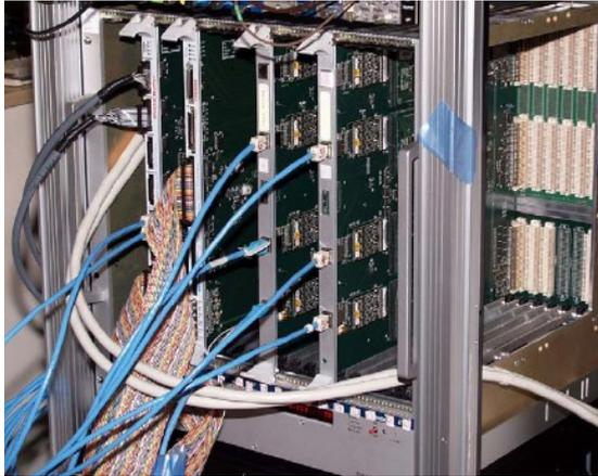
**Figure 5:** Picture of the VME crate housing the DAQ boards: NECO, Buffer and two FADC boards.
