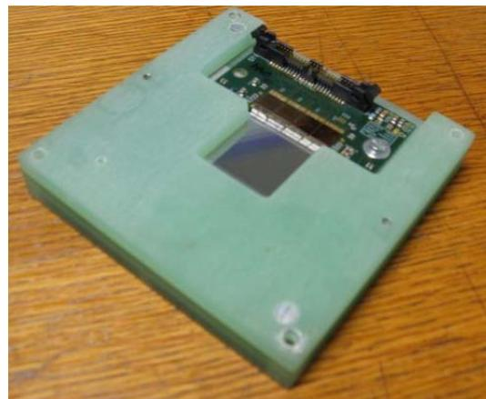
**Figure 3:** Quadratic baby sensor, p-side up.
