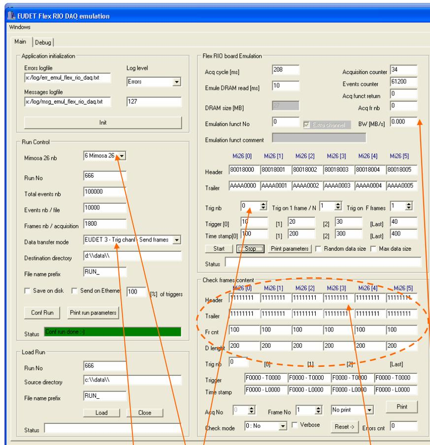
Emulator in mode **EUDET 3**, **6 Mimosa 26**, **default frame size**, **no trigger**, **frame No 0 has a strange pattern** and bandwidth field indicates 0 !
