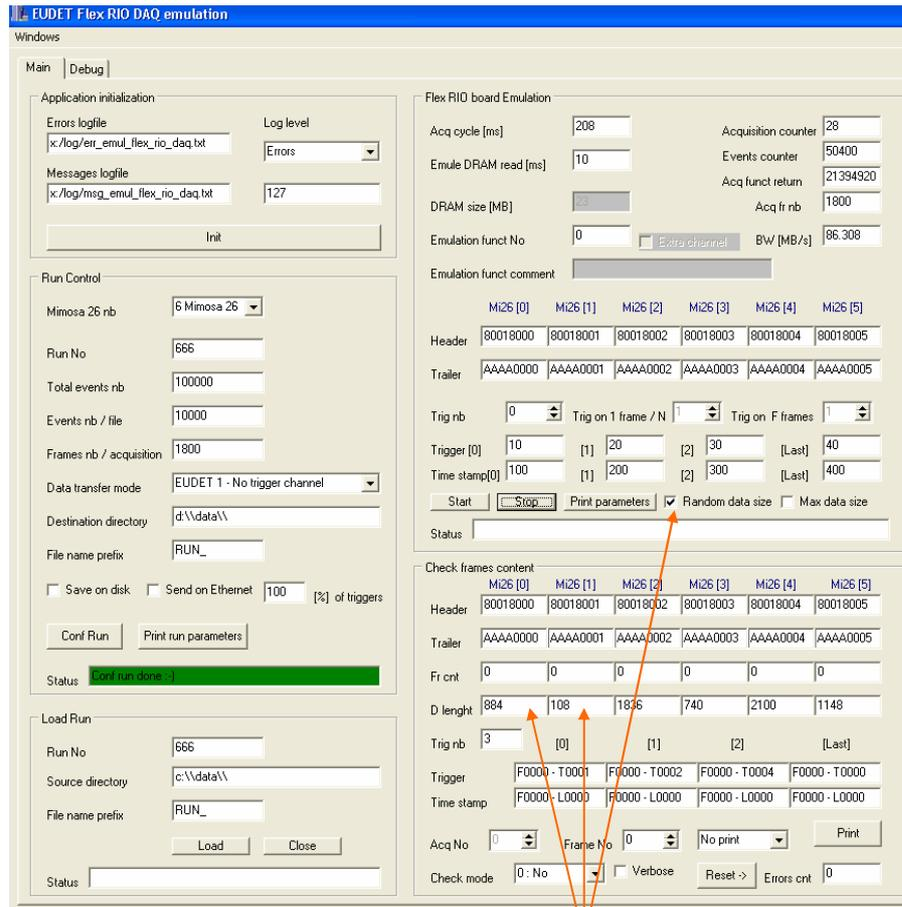
Emulator in mode EUDET 1, 6 Mimosa 26, random frame size, three trigger are generated and frame No 0 is displayed.
