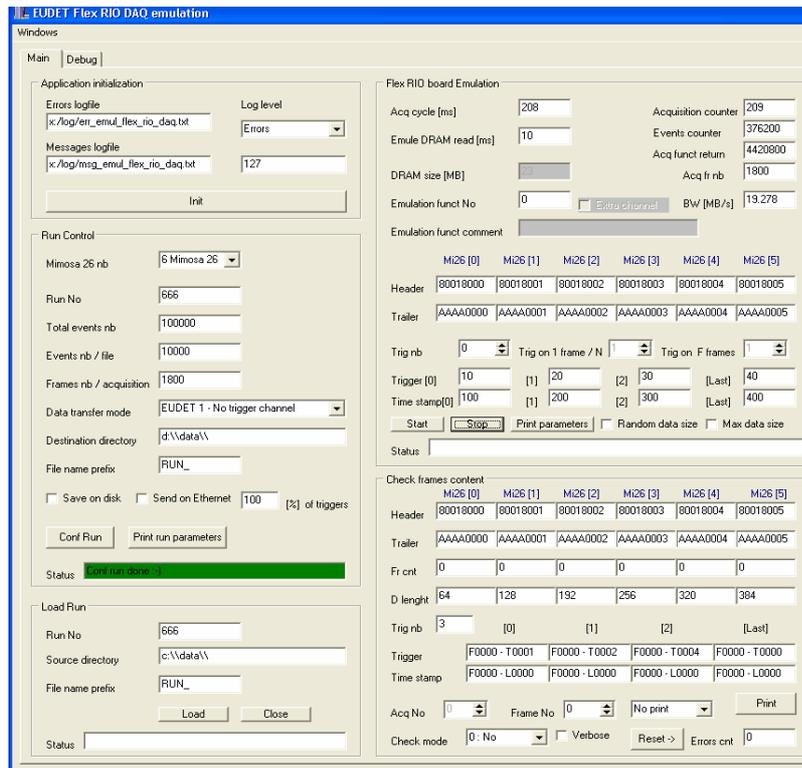
The emulator can also allow you to **measure functions execution time** by generating a **pulse on PC parallel port** during their execution. If you want to **run the software in this mode**, you need to **compile it with parallel port enabled** (the conditional compilation directive **EFRIO\_INCLUDE\_PARA\_PORT** must be enabled in file **app.def**) and to run it via the **a batch file** names : **run emul\_flex\_rio\_daq.bat**.
