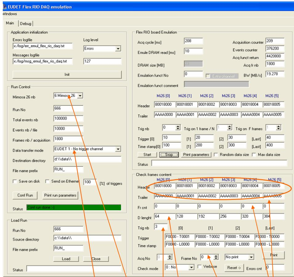
Emulator in mode EUDET 1, 6 Mimosa 26, default frame size, three trigger are generated and frame No 0 is
