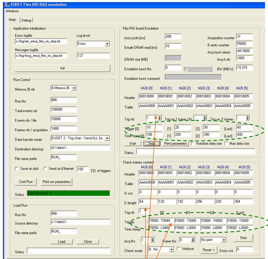
Emulator in mode **EUDET 2**, **6 Mimosa 26**, **default frame size**, **one trigger generated** and **frame No 0** is displayed.
