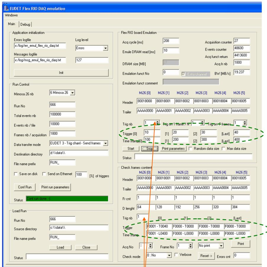
Emulator in mode **EUDET 3**, **6 Mimosa 26**, **default** frame size, **one trigger generated** and **frame No 0** is
