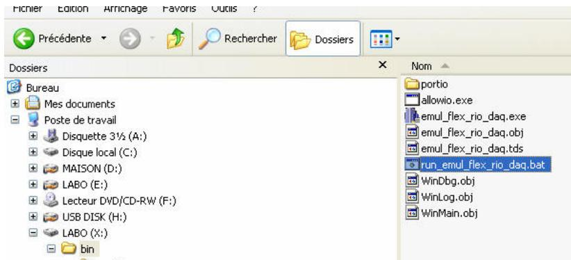
**If, by mistake, you run the version compiled with PC parallel port handling directly via a call to executable file ( not via the batch ) you will get exception errors. Because access to parallel port is not allowed, please kill the program and start it via batch file.**
