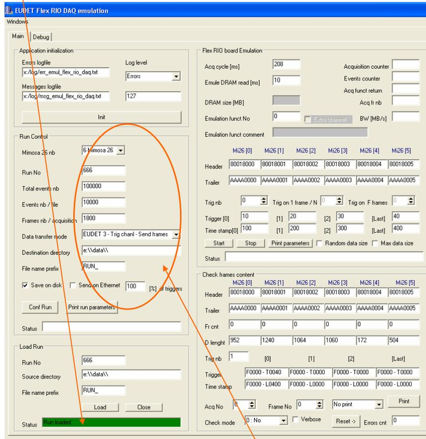
The run parameters, of the loaded file, are displayed in “ Run Control ” panel.
