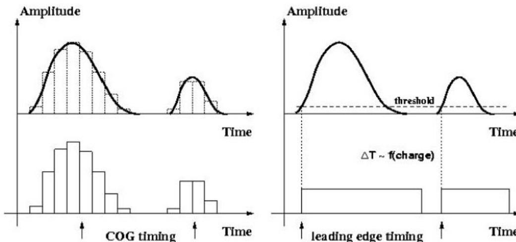
Figure 7: Principle of TDC based electronics. In contrast to the ADC based readout (left) the charge of the input signal is encoded into the width of the pulse (right).
