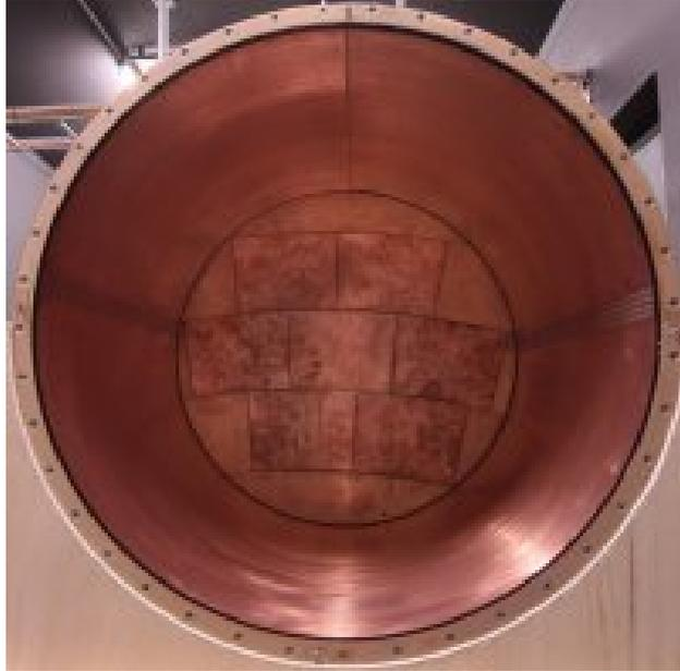
Figure 1: The LP field cage. On the back side one can see the inner part of the anode end plate equipped with seven dummy modules.
