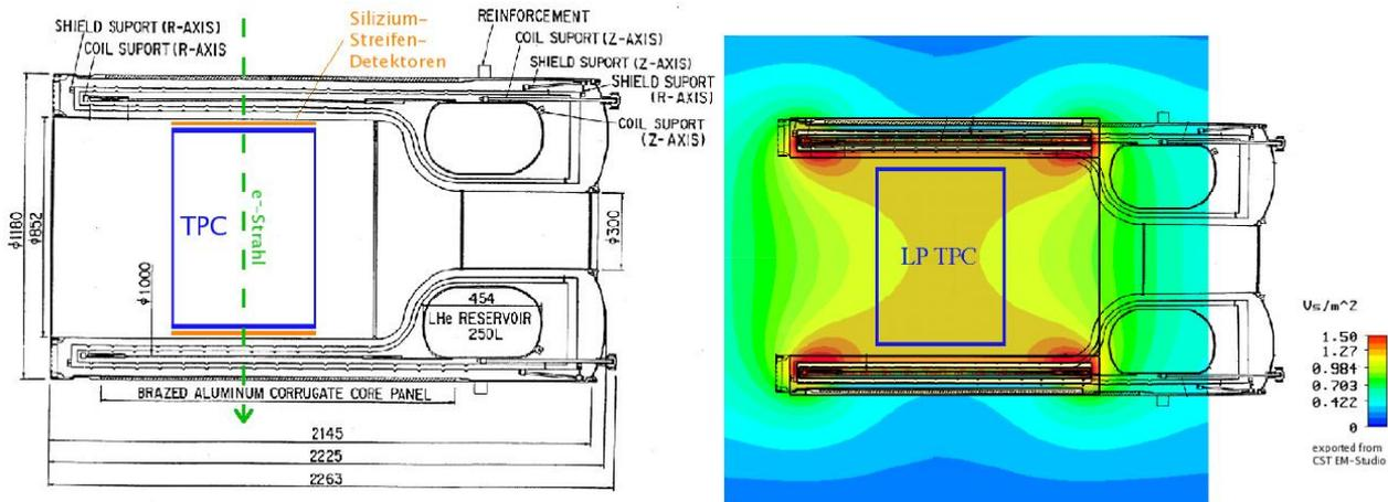
Figure 9: Schematic drawing of PCMAG and its field density distribution.
