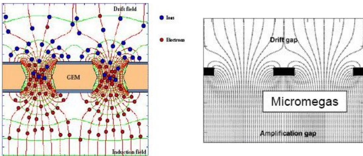
Figure 4: MPGD techniques. Left: GEM, right: MicroMegas.
