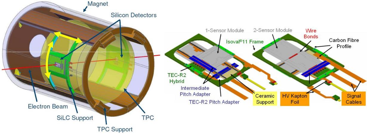
Figure 8: Silicon detectors which are mounted on a support structure around the LP (left) and a zoom in of the Si-modules (right).
