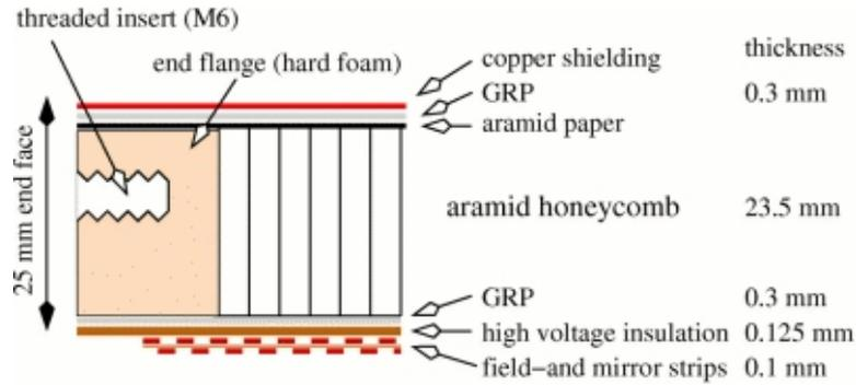
Figure 2: Sandwiched structure for the field-cage.
