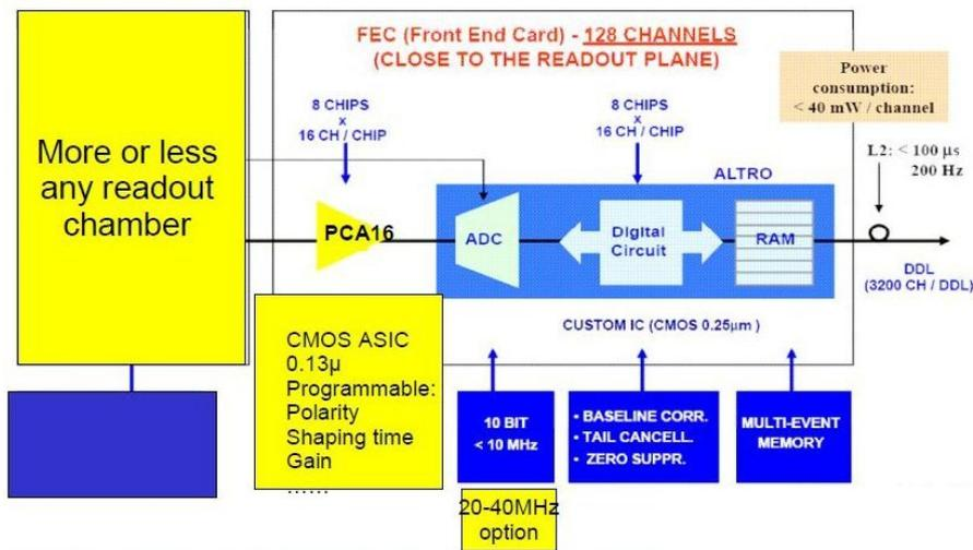
Figure 6: Schematics of the ALTRO electronics. The PASA chip has been replaced by the PCA16 chip. The AFTER electronics which will be used for the MicroMegas modules have a similar setup.
