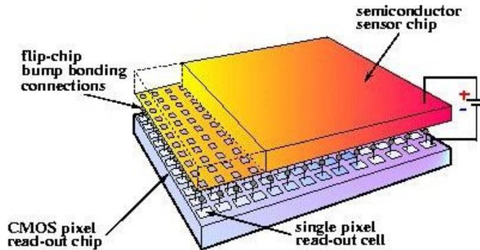
Figure 5: TimePix readout technique.
