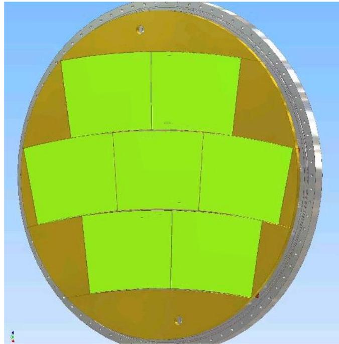
Figure 3: Schematics of the anode end plate with amplification modules and termination plates.
