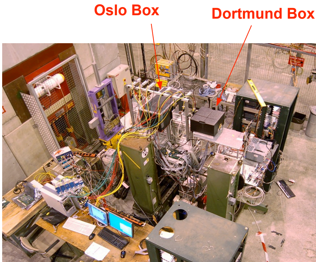
Figure 2: The EUDET telescope during the ATLAS Pixel test. Up to 8 DUTs were placed into the system, 4 in the Oslo box between the two telescope arms, another 4 in the Dortmund Box behind the telescope. 2
