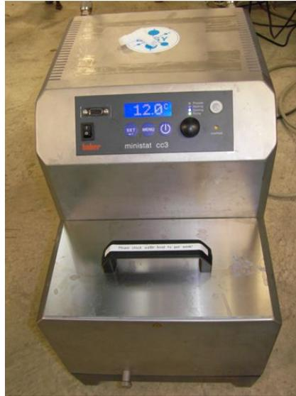
Figure 6: The Huber cooling device
