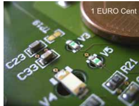
Fig. 2: Assembled UV LEDs (V3, V5) of the proposed calibration system.
